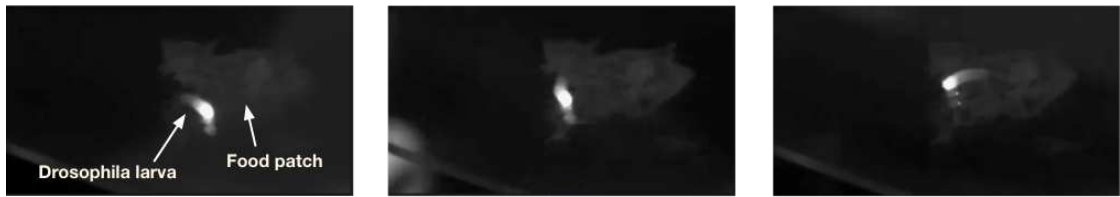
Figure 8.6: Images of the Drosophila larva illuminated by the tracking beam, collected using the camera C. As the larva moves around the glass slide it remains illuminated by the tracking beam locked onto a feature just above its heart.
