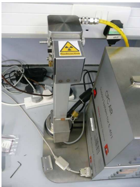
Figure 4.1–8. Grimm SMPS. Aerosol input can be seen at upper left. For this calibration the neutraliser attached to the top of the DMA (displaying the radioactive symbol) is removed.
