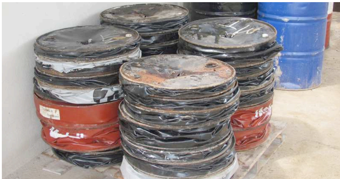
Fig. 6.3: Crushed waste oil drums, prior to their safe disposal. Source: Zeal Environmental Tech. Ltd.
