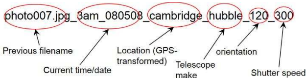
Fig.6 A multi-dimensional search in a traditional filesystem can be performed by changing the filename format as a concatenation of the selected attributes.
