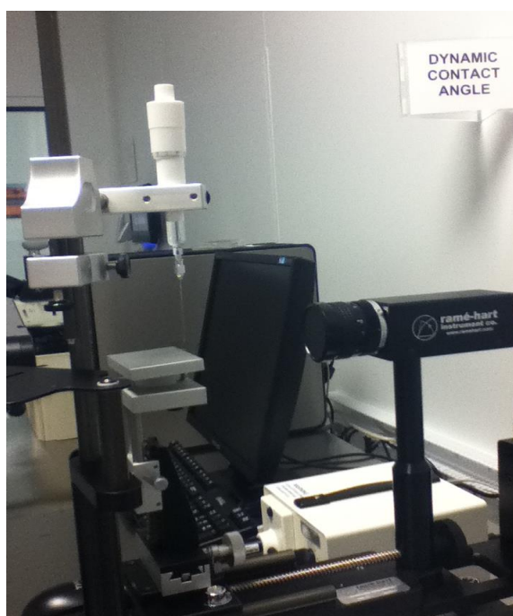
Figure 6-2: Contact Angle measurement instrument in the Marcus Nanotechnology Centre at GeorgiaTech (Ramé-Hart, USA)
