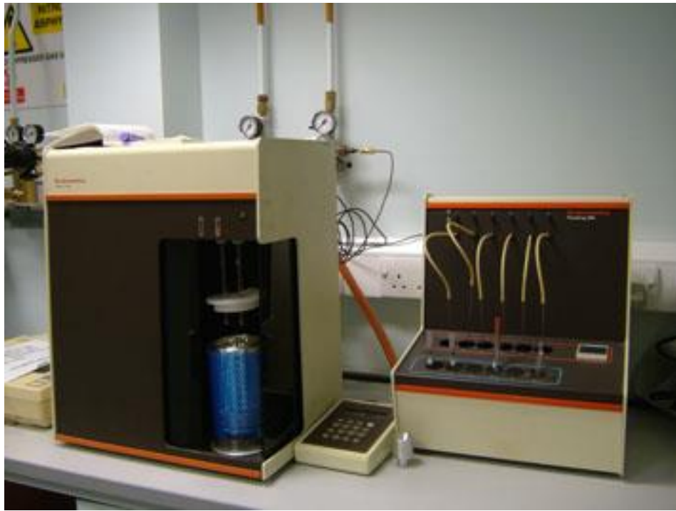
Figure 2-20: Instrument for the determination of surface area by BET in the IRC centre at QMUL (Micromeritics, UK)
