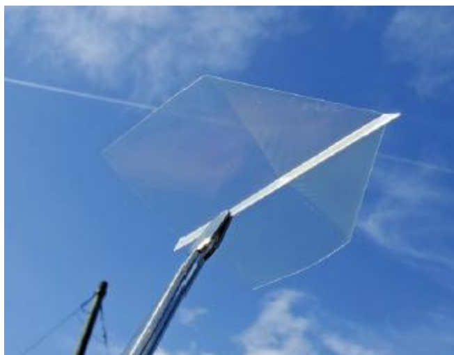
Figure 3.18. Foldable optically transparent nanpaper 148 .
