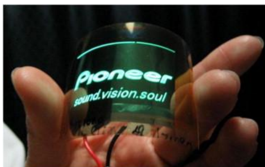
Figure 3.16. Luminescence of an organic light-emitting diode deposited onto a flexible, low-CTE and optically transparent wood–cellulose nanocomposite 144 .
