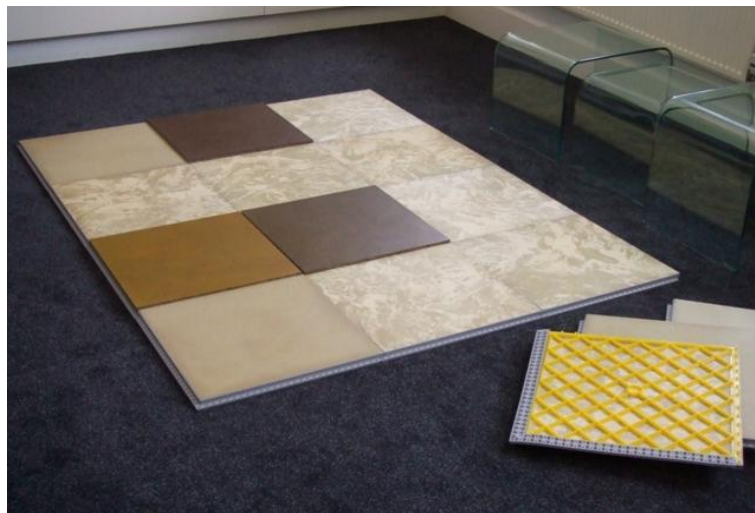
Figure 1.2. Binder-free all-cellulose composites for flooring application.
