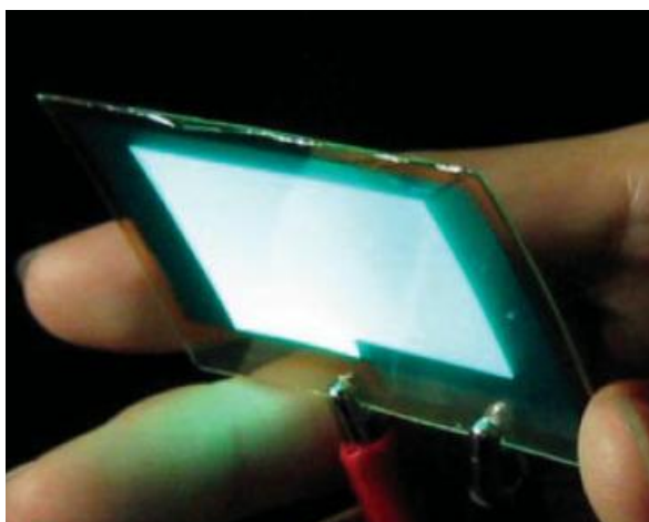
Figure 3.20. Luminiscence of an OLED deposited onto a transparent BC nanocomposite 151 .
