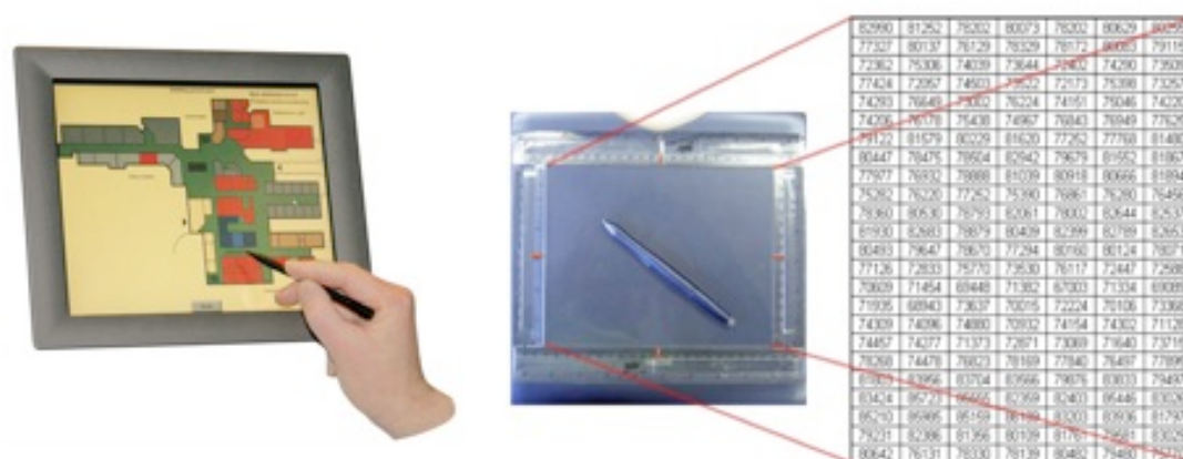
Figure 14 pin Tablet displays, a diagram overlay left, and a numerical data table right, auditory feedback is display when the users touches parts of the tablets with a stylus
