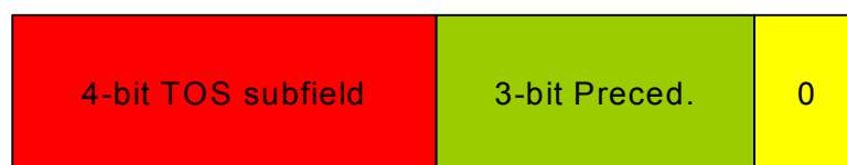
Figure 2.2. IP Type of Service Field
