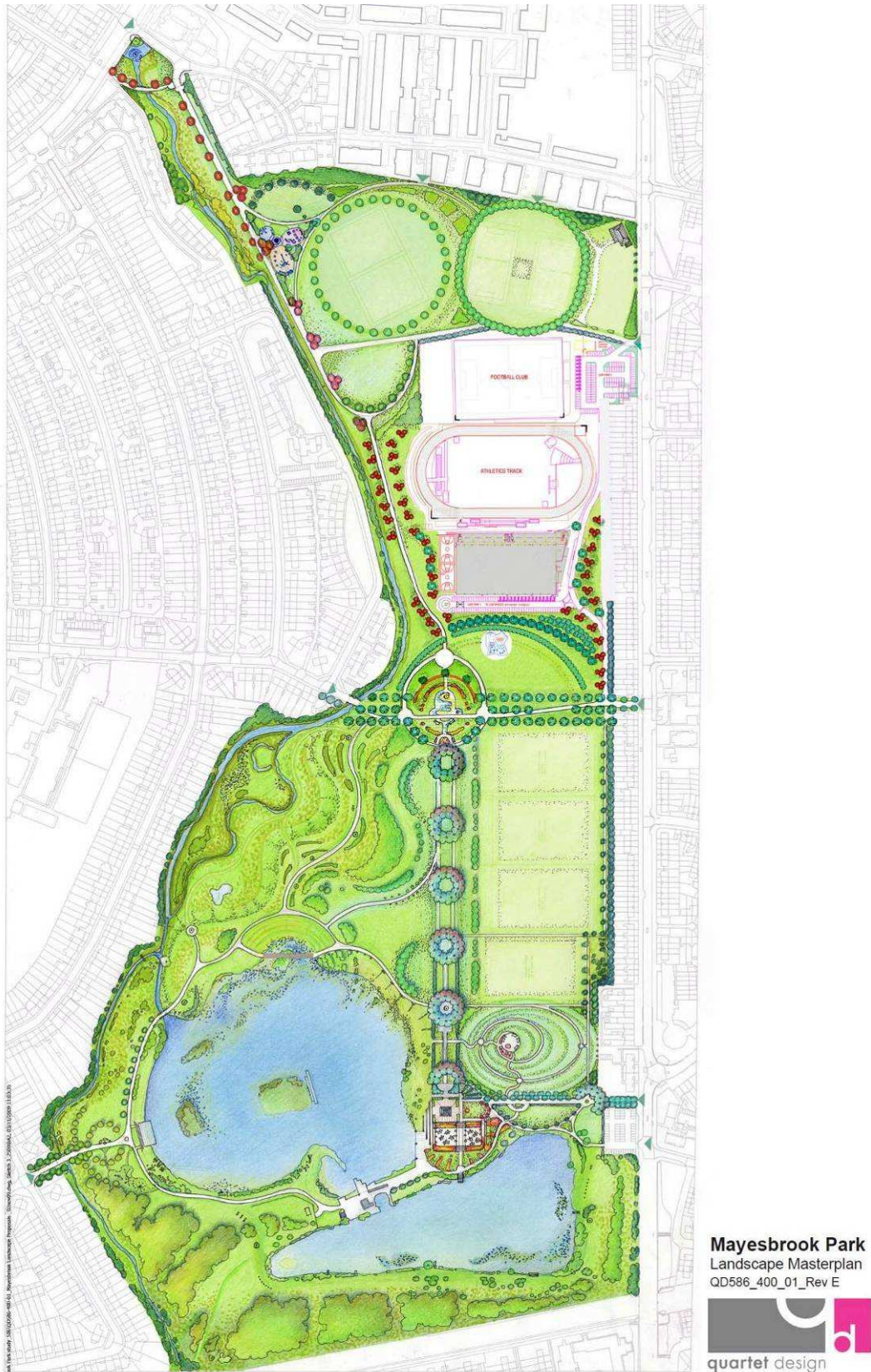
Figure 6.22 Masterplan document: Design of new brook channel and surrounding parkland. Source: Quartet Design, 2009c.
