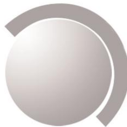
Figure 6.1: Cup diameter much larger than head diameter, which can result in a small contact area [adapted from Wright Medical, 2007]
