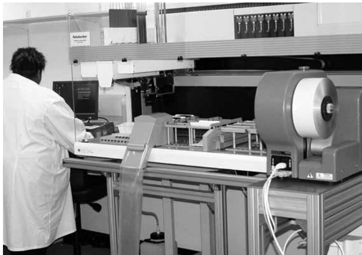
Figure 10. Robobanker robot. In 2003, ALSPAC acquired two robots to immortalize cell lines. They were named by cohort members, the ‘Germinator’ which grew cells and ‘Robobanker’ (pictured) which stored them.
