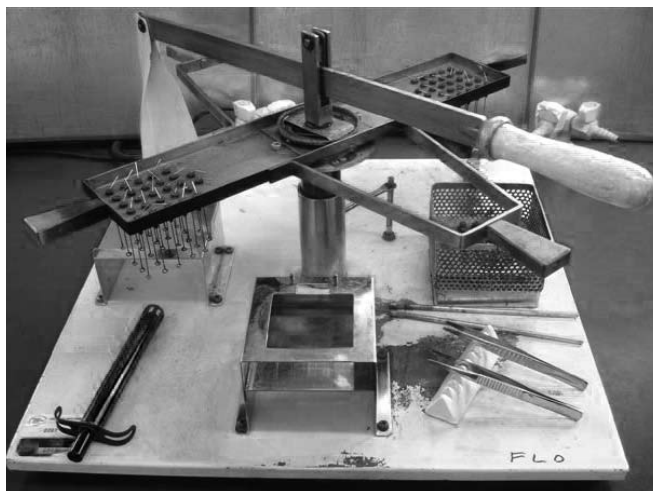
Figure 13: Lidwell 'phage typing machine used in the Staphylococcus Reference Laboratory for almost 50 years. 176
