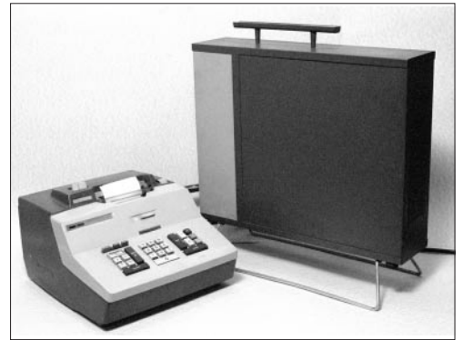
Figure 53: Litton Monroe Epic 3000 keyboard and printing unit with free-standing calculating unit, introduced in 1967 as the first programmable printing calculator. © Nigel Tout.
