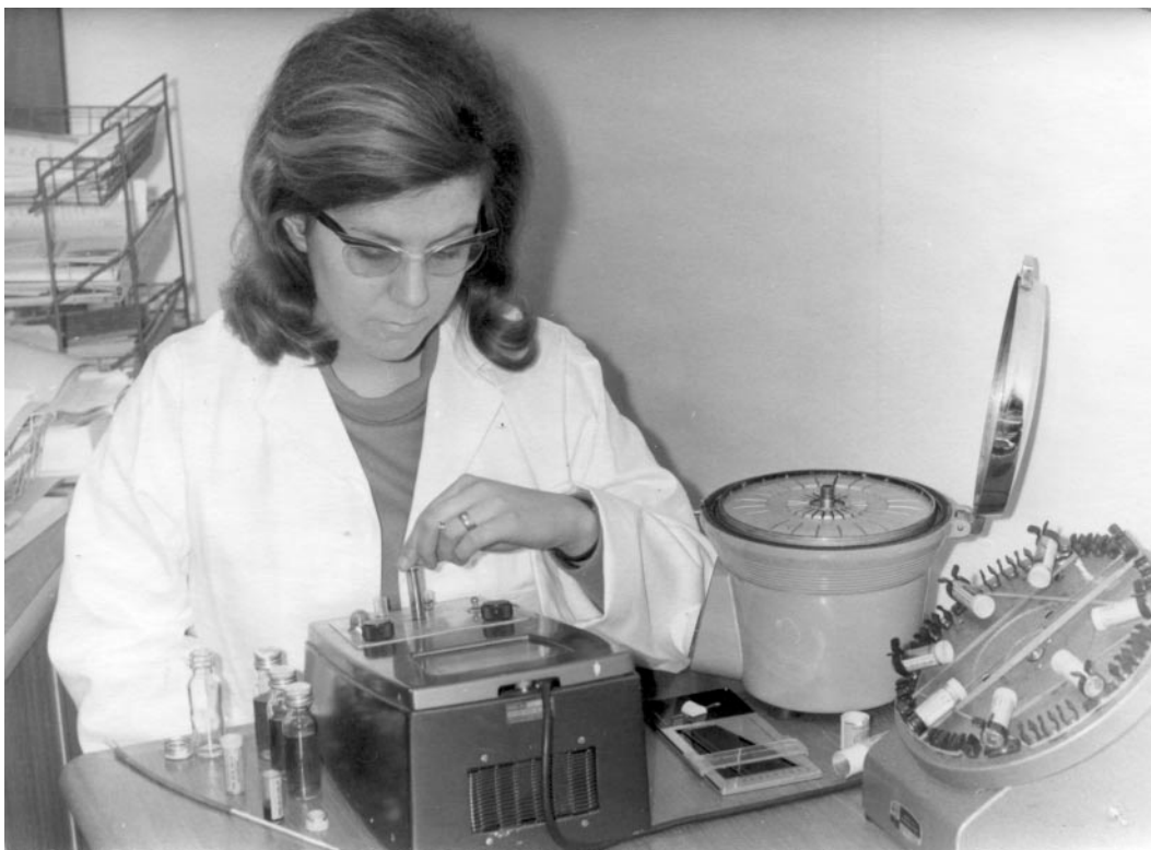
Figure 48: Janie Hughes testing haemoglobin (Hb) levels on a haemoglobinometer, 1967.
