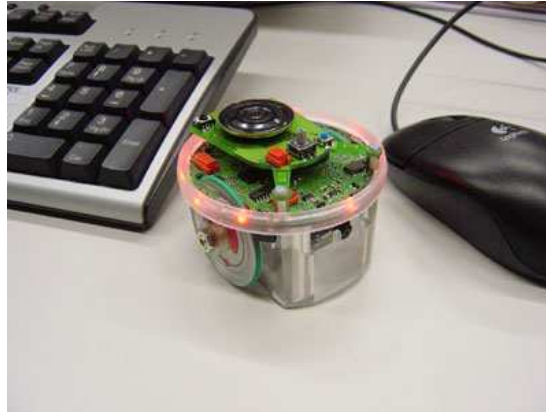
Figure D.1: E-Puck robot. Photo from (Mondada and Bonani, 2007).
