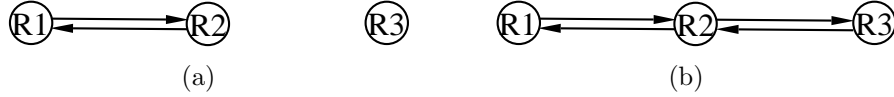
Figure 3.1: Communication graph structures used in simulations: (a) disconnected graph (b) connected graph.
