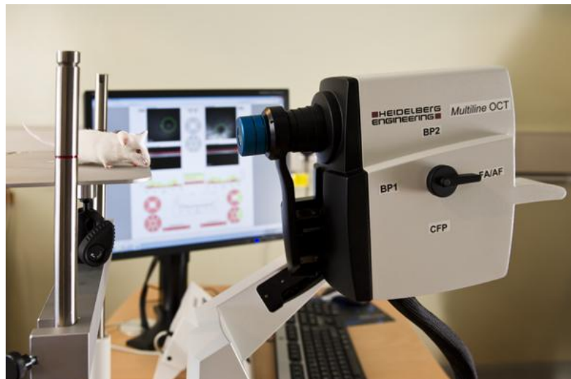
Figure 5.2 Setup of Multiline OCT. A Spectralis HRA + OCT from Heidelberg Engineering was modified to allow imaging of MOG TCR xThy1CFP mice.
