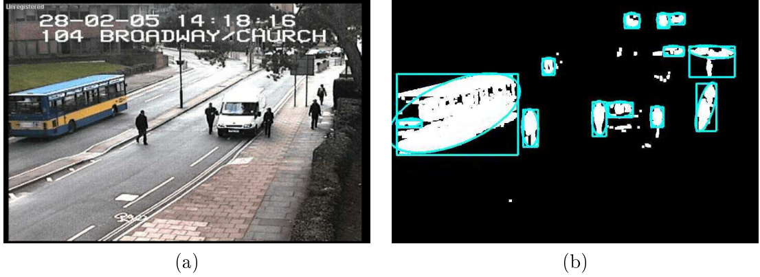
Figure 3.8: Illustration of the fit of ellipses to blobs with a fit measure and a maximisation algorithm. (a) The original image. (b) Fitted ellipses to each object blob as outputted by the moving object detection process. The four dimensional tracker uses the bounding boxes as detection input, whereas the five dimensional code uses the ellipses.
