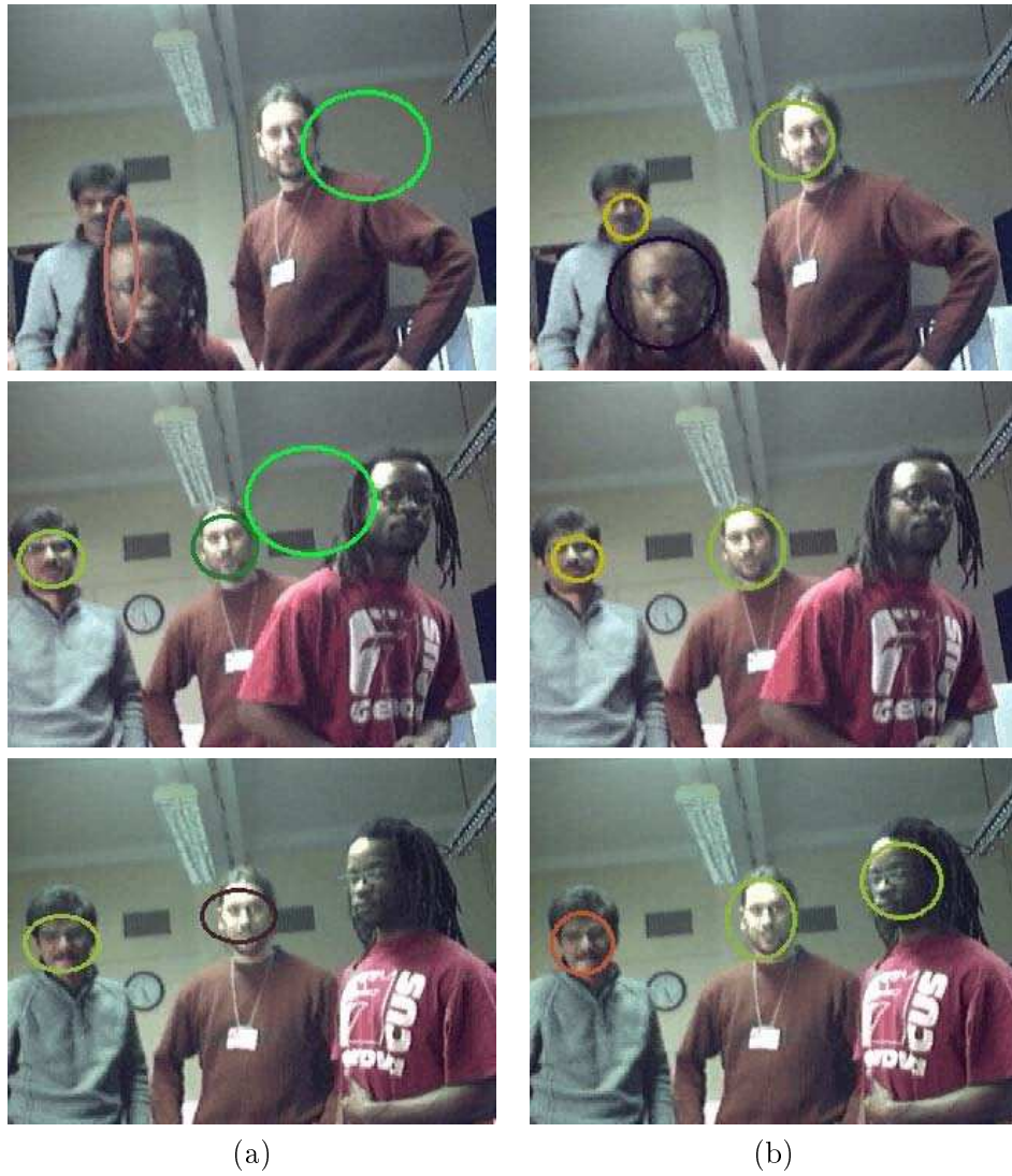
Figure 3.10: Illustration of limitation of particle filtering using the detector for initialisation only. (a) Tracks lost without integration of the detector with the particle filtering state estimation. (b) Better results with integration.
