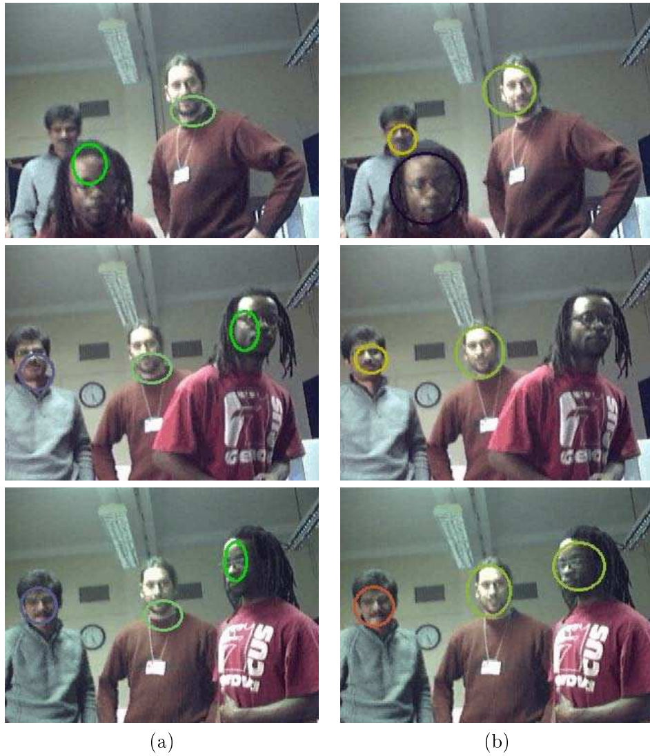
Figure 3.11: Illustration of limitation of particle filtering without update of the the colour model. Without update of the colour histogram model state estimation is unsatisfying (a) however with update (b) state is accurately estimated.
