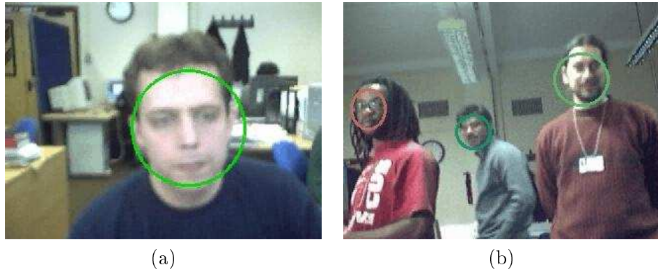
Figure 3.17: Example tracks generated by the face tracker for (a) one face and (b) three faces.
