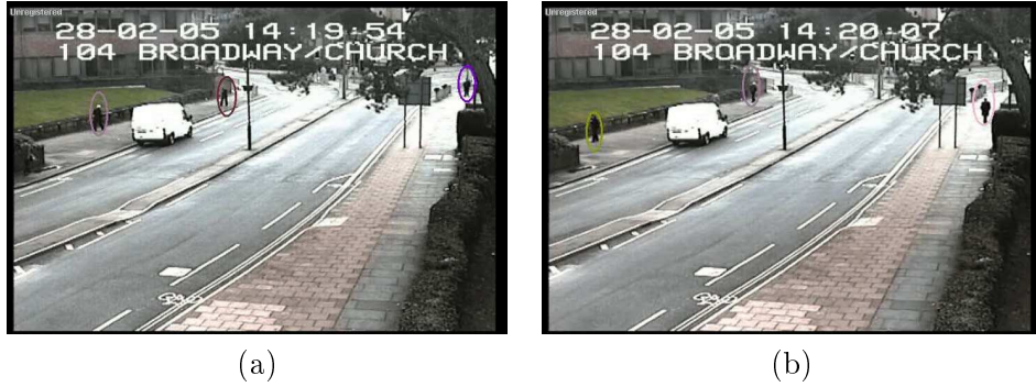
Figure 3.24: Example frames of successful people tracking. The people detector fails to estimate the size of the person in many cases, which results in too large target ellipses.
