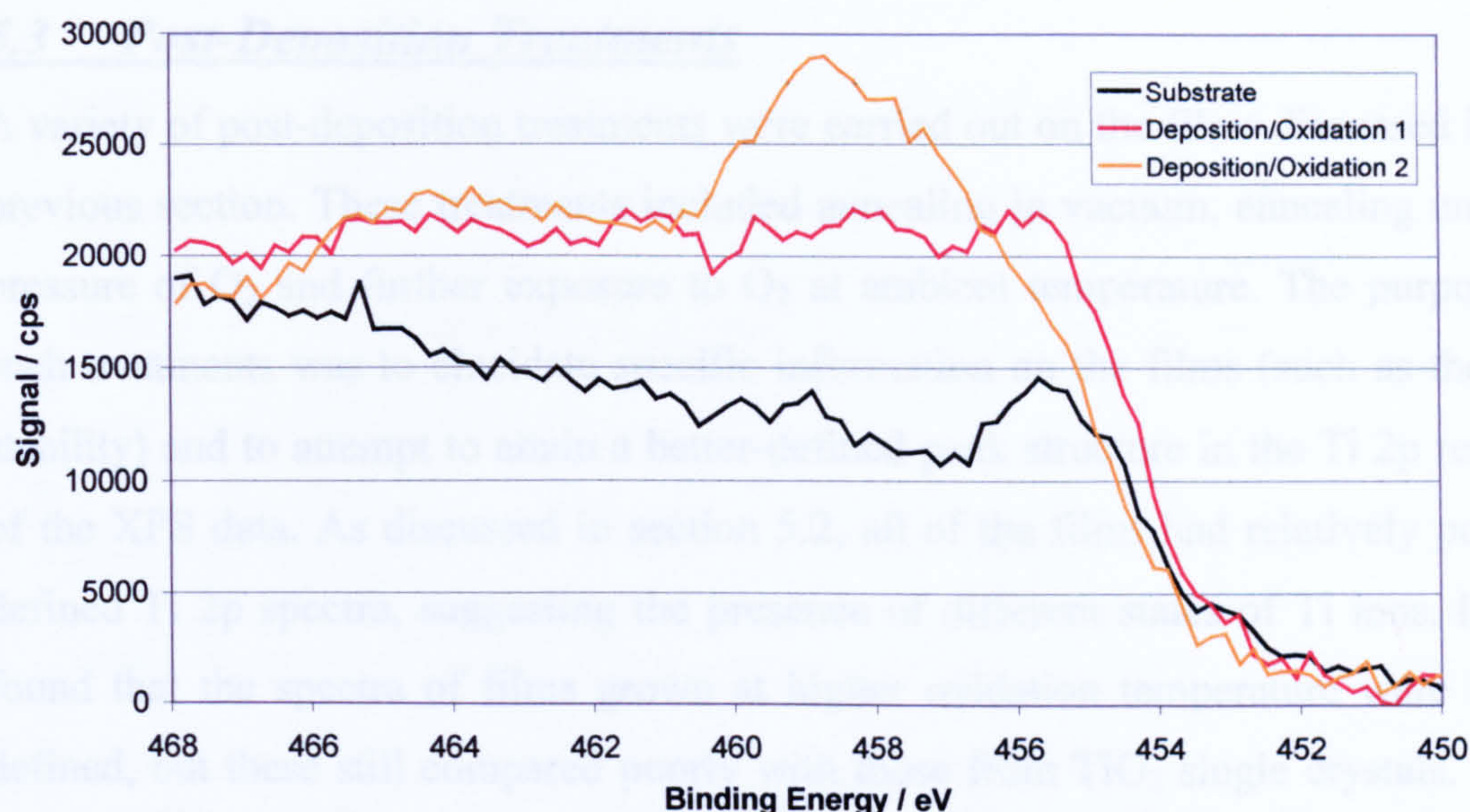
Figure 5.10: Ti 2p region for growth of film F (Deposition/Oxidation = after deposition of Ti metal for 2 mins whilst exposing to 24 L \text{O}_2 at 673 K)
