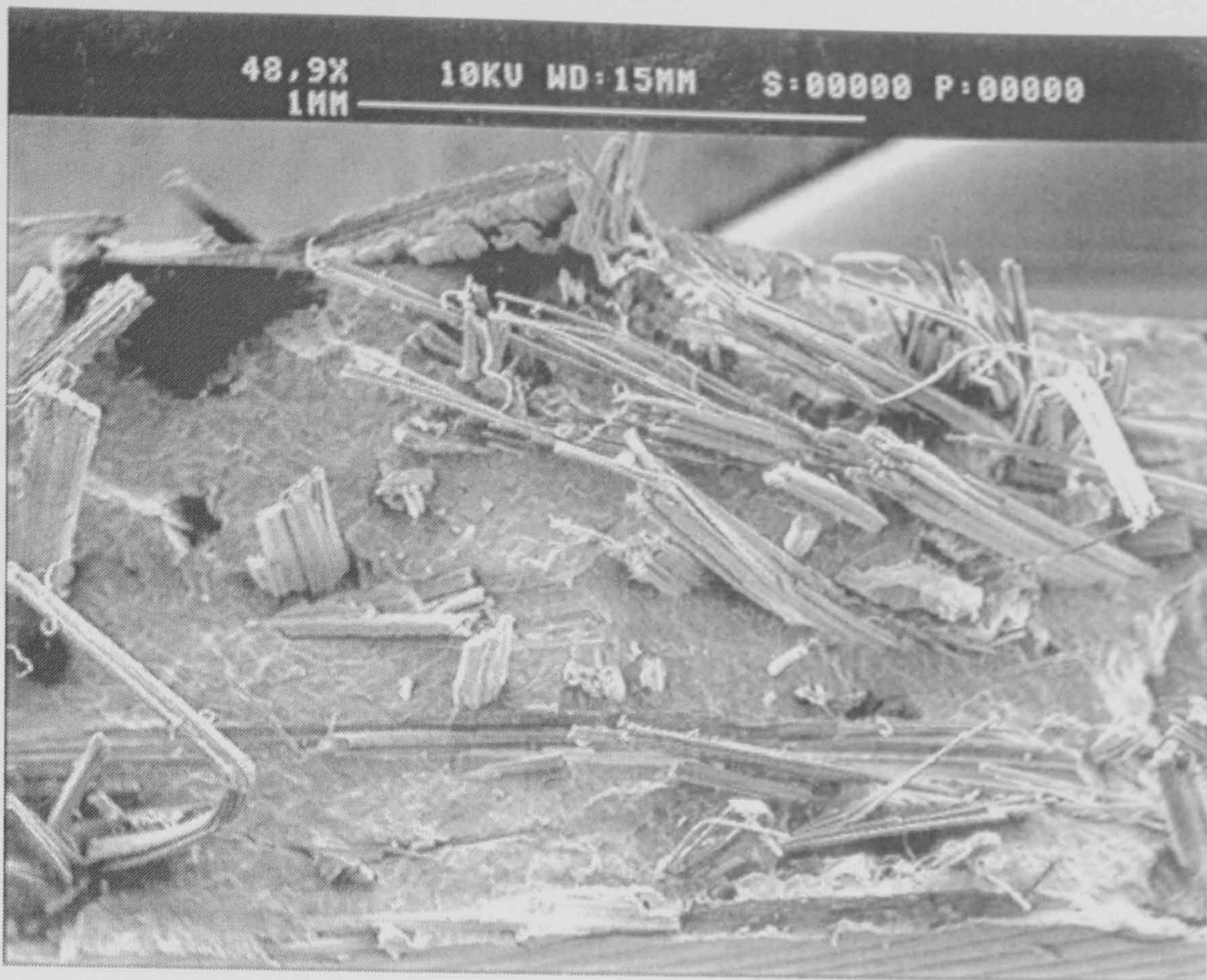
Figure 5.6 Scanning electron micrograph of fracture surface of flax/MA-PP composite ( V_f=0.2 and fibre length = 25 mm).
