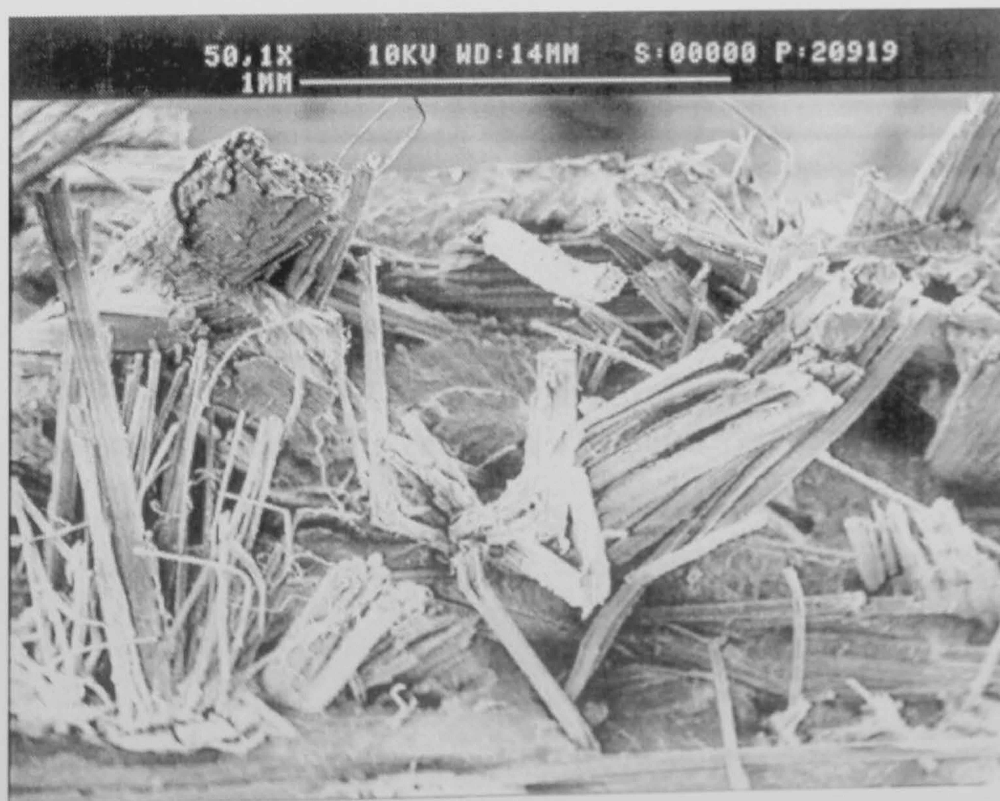
Figure 5.5 Scanning electron micrograph of fracture surface of PP/flax composite ( V_f=0.2 and fibre length=25 mm).
