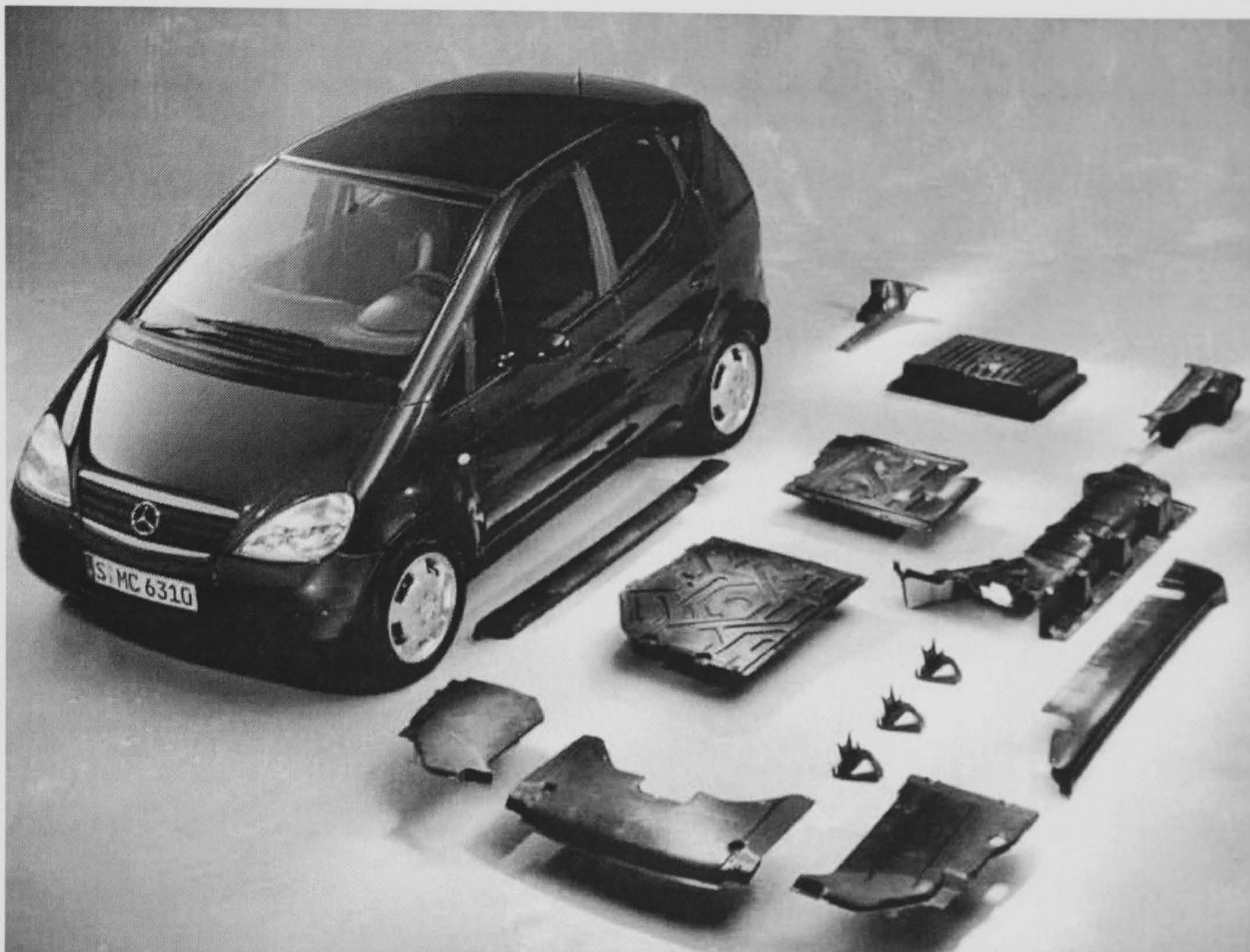
Figure 1.10 Underbody panelling prototypes for the Mercedes A-class made of flax-fibre-reinforced polypropylene (photo courtesy Daimler-Chrysler).
