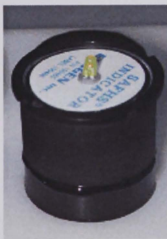
FIGURE 3.4: LED indicator placed on transducer with coupling gel. The LED glowed yellow when PLIUS was transmitted.
