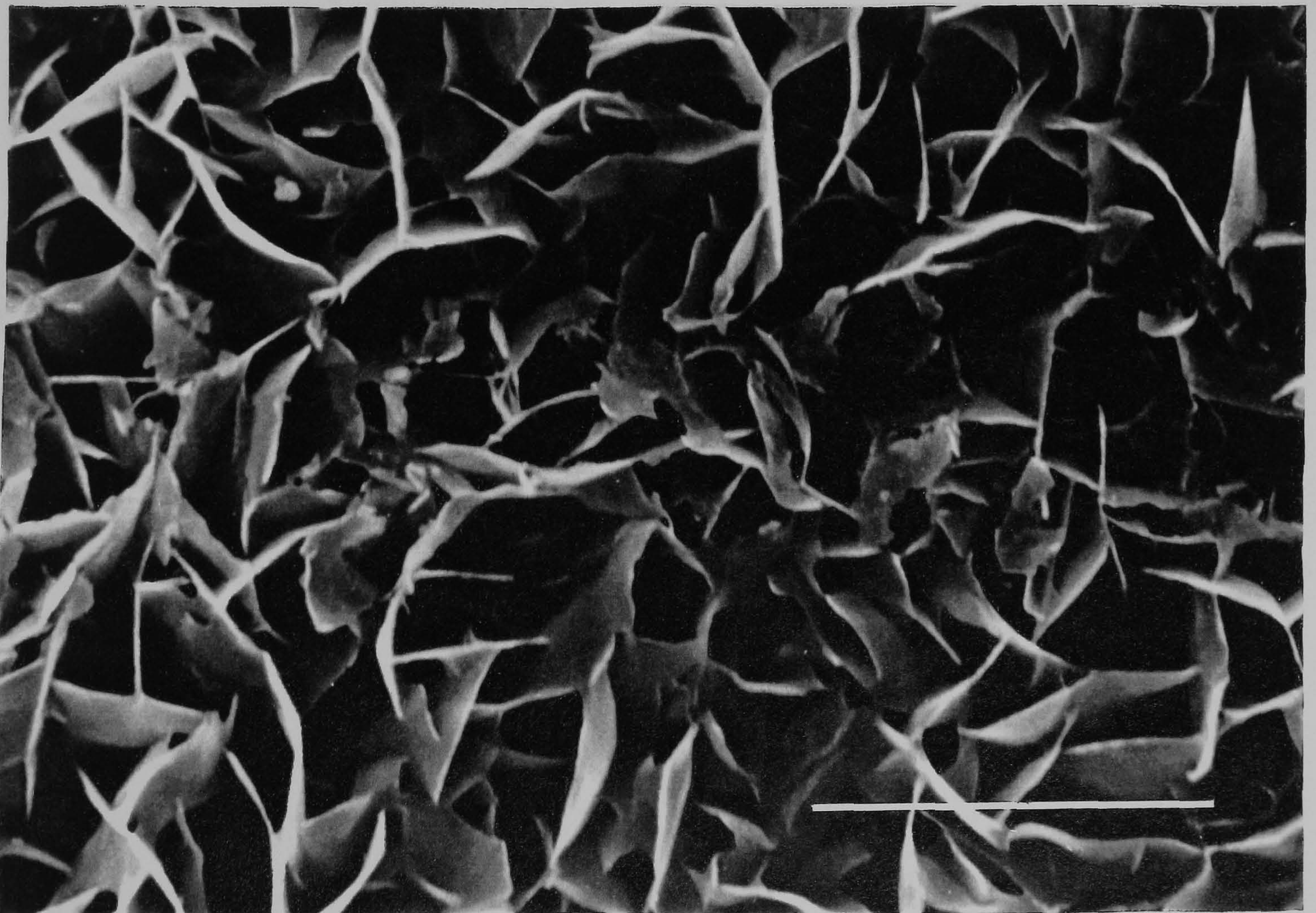
Figure 3.5 Scanning electron micrograph of a CdS film as grown on glass for 2 hours, [\text{Cd}] = 0.018 \text{ mole dm}^{-3} , [\text{thiourea}] = 0.018 \text{ mole dm}^{-3} at 40^\circ \text{C} , \text{pH} = 10.2 , [\text{Cd}]:[\text{en}] 1:2.5 , ----- = 1 \mu .
