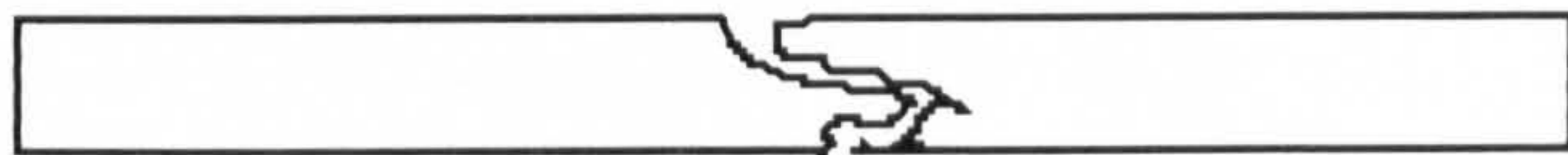
Fig. 6.26 Flexural test failure types of specimens moulded at different ranges of temperature for the CDMC with AR50/1 glass or E-glass.
