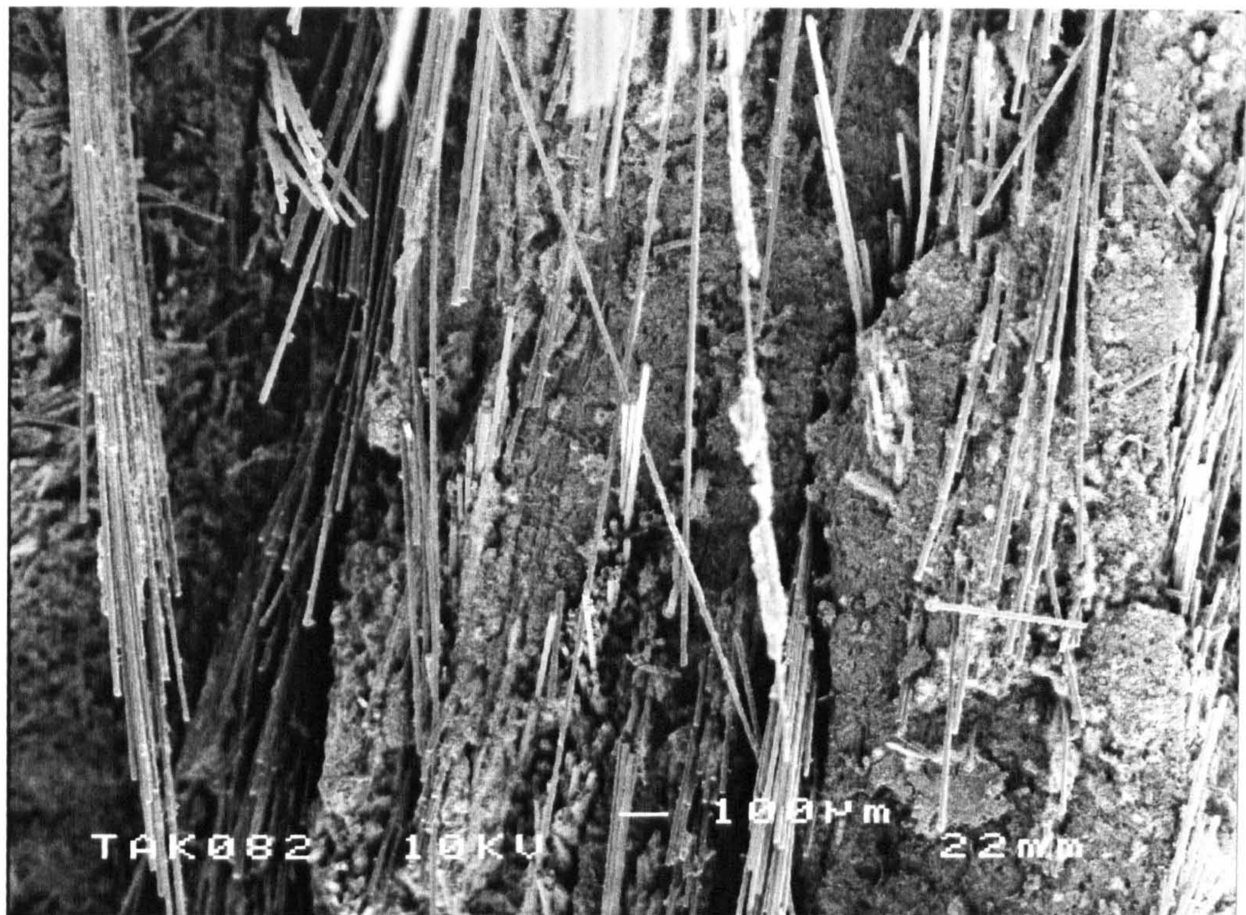
Fig. 6.28 The SEM micrograph of a flexural fracture surface, specimen moulded at 99 °C, the CDMC with 22.6%(vol.) AR-glass fibre. Some fibres were pulled out completely.
