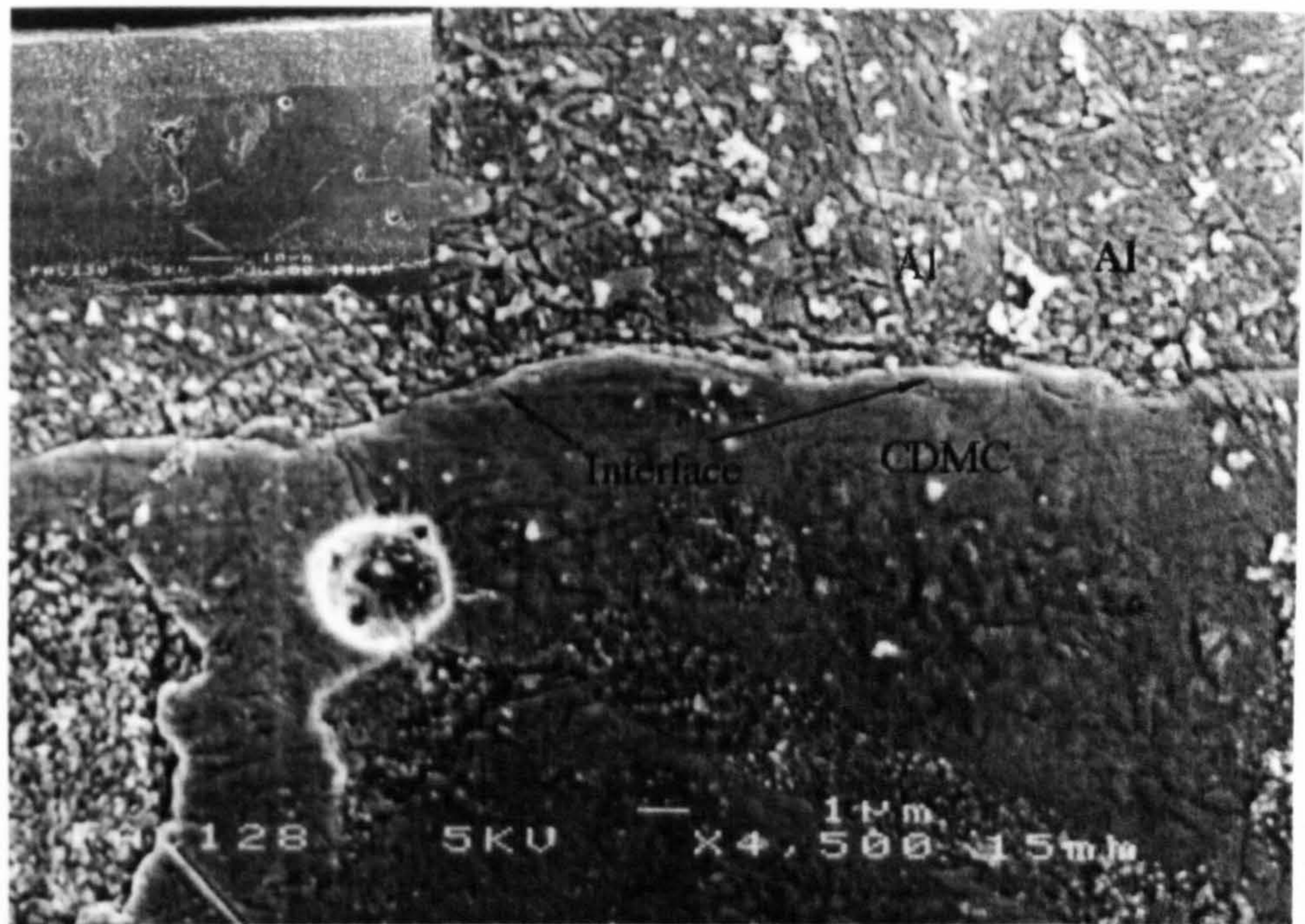
Fig. 9.4 The interface between the ceramic matrix and Al foil, shows a good bonding. The heat shields without environmental tests generally presented good interface.
