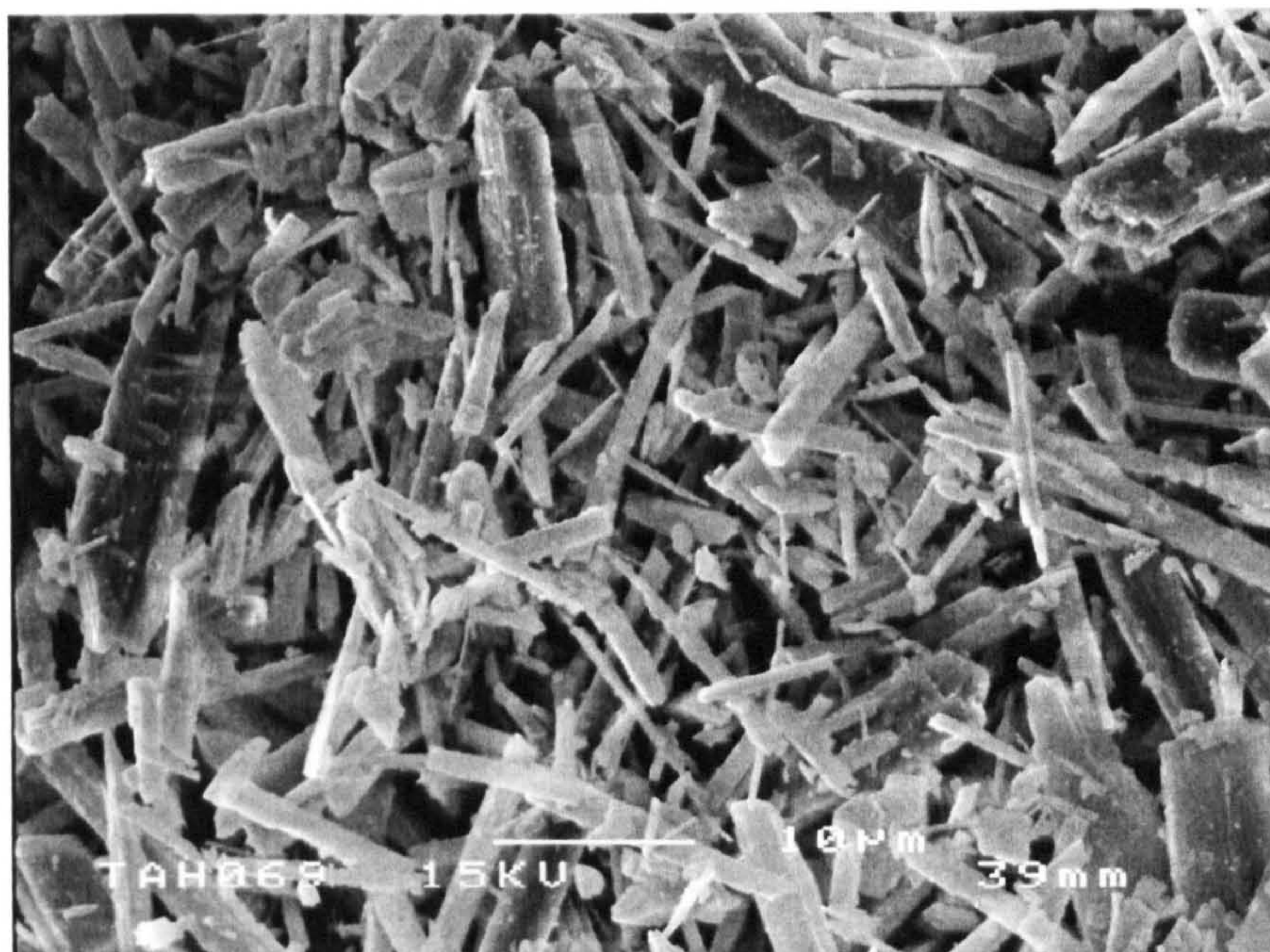
Fig. 4.11 A SEM micrograph of the fibrous Wollastonite.
