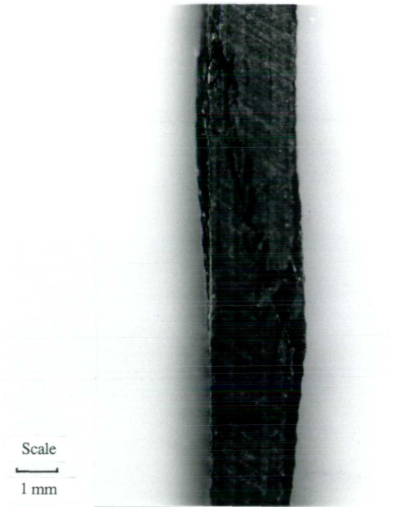
Fig 7.2 Shear type failure at edge of specimen after impact and compression testing. Spec No 41/2. Incident Impact Energy 0.96 J. TCE-QI-16-55.
