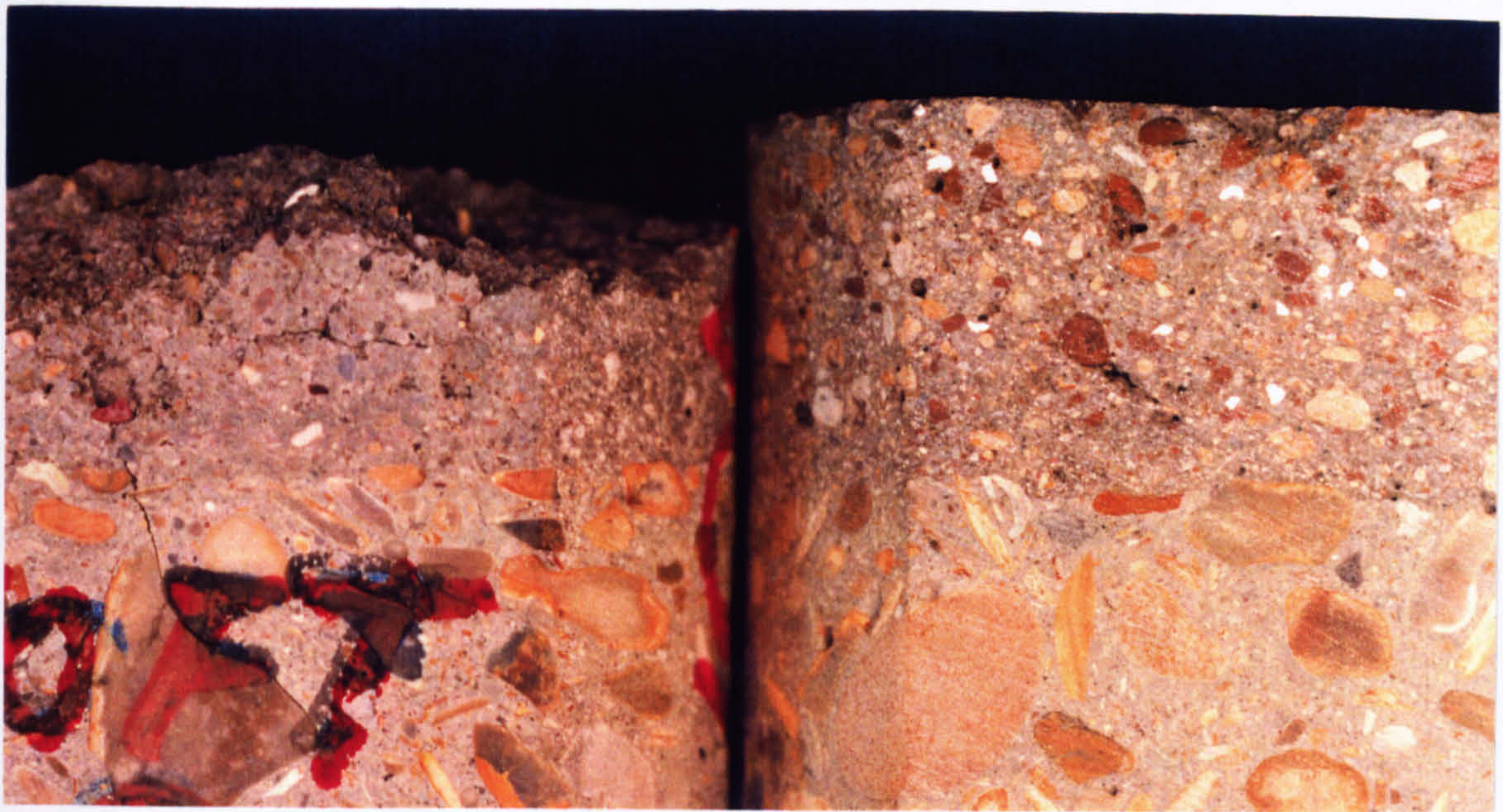
Figure 8.4 - Normal mix sprayed concrete tested (left) untested (right)
