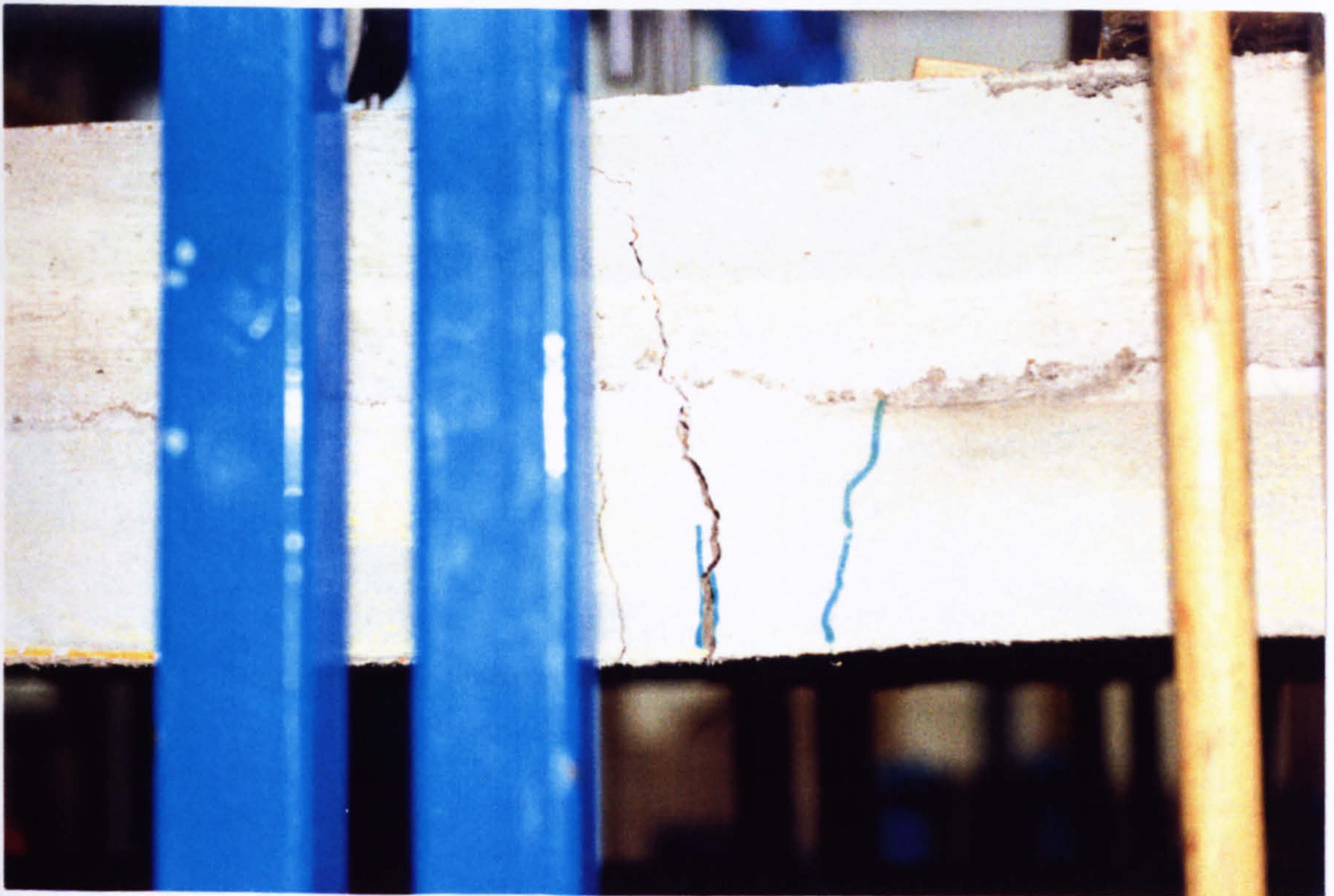
Figure 4.17 - Ductile failure of test slab A5.
