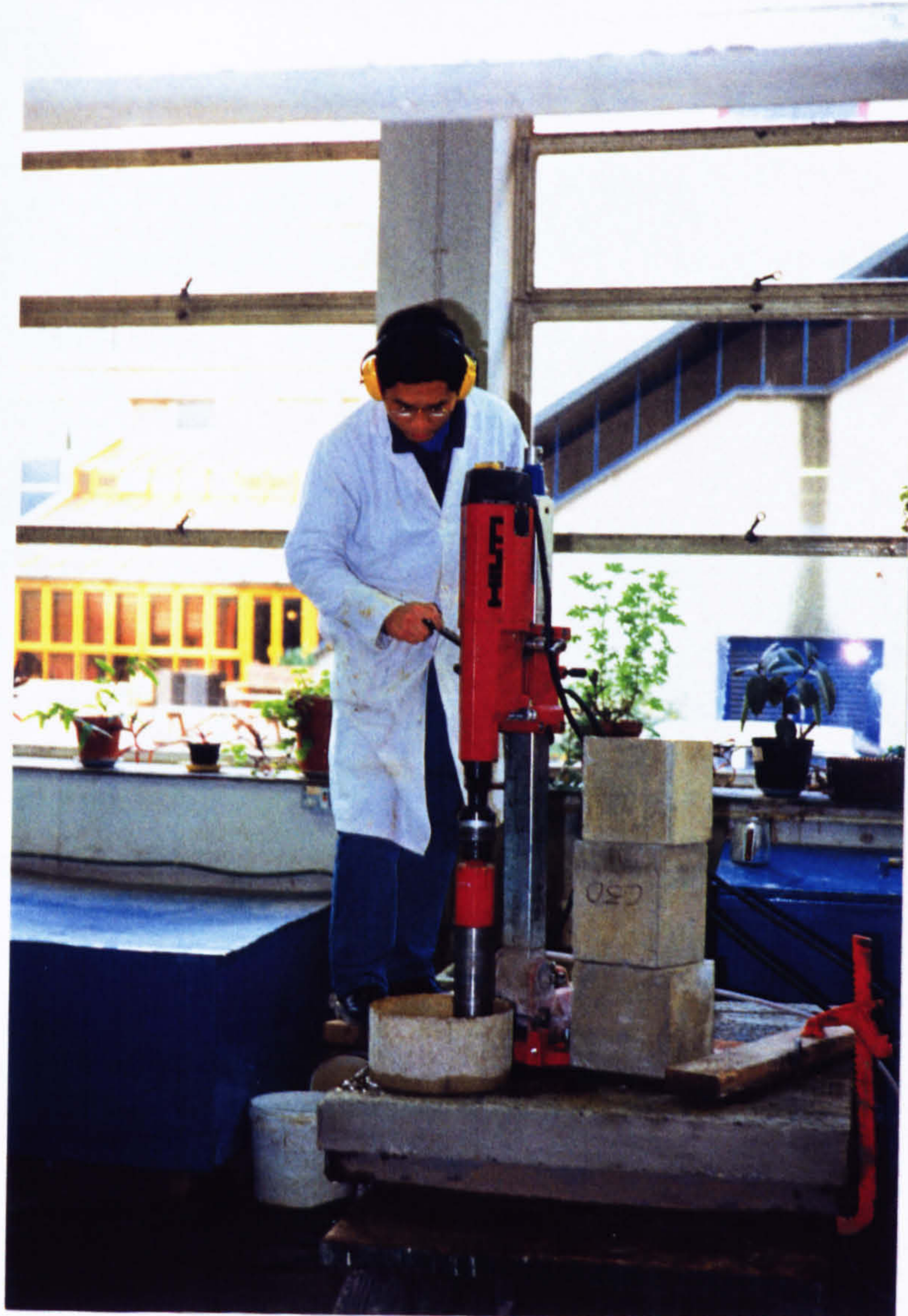
Figure 7.6a - Through-Drilling to extract cores.
