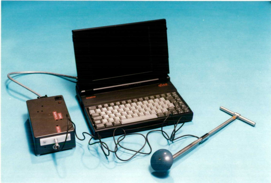
Figure 3-23: The instrumented acetabular cement pressuriser and recording apparatus.
