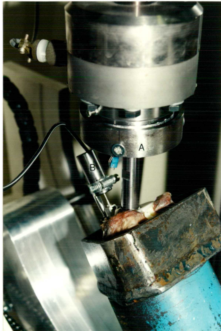
Figure 6-9: Potted acetabulum ready for testing.
