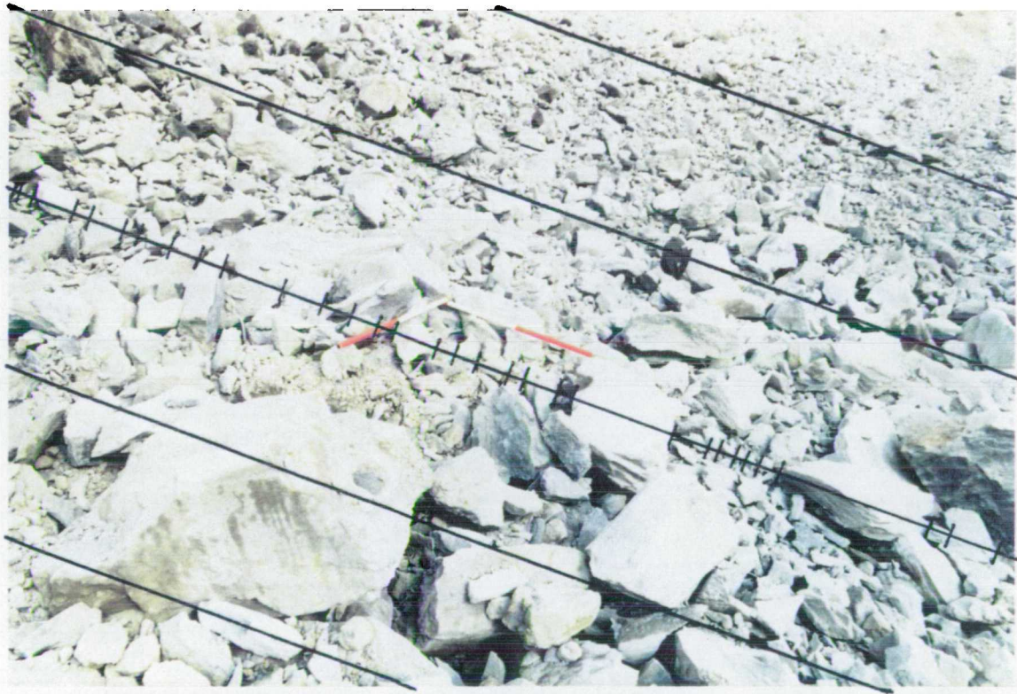
Fig. 5.1 Schematic illustration of the photo-scanline technique (the scale rod in the centre of the photograph has a 50 cm division).
