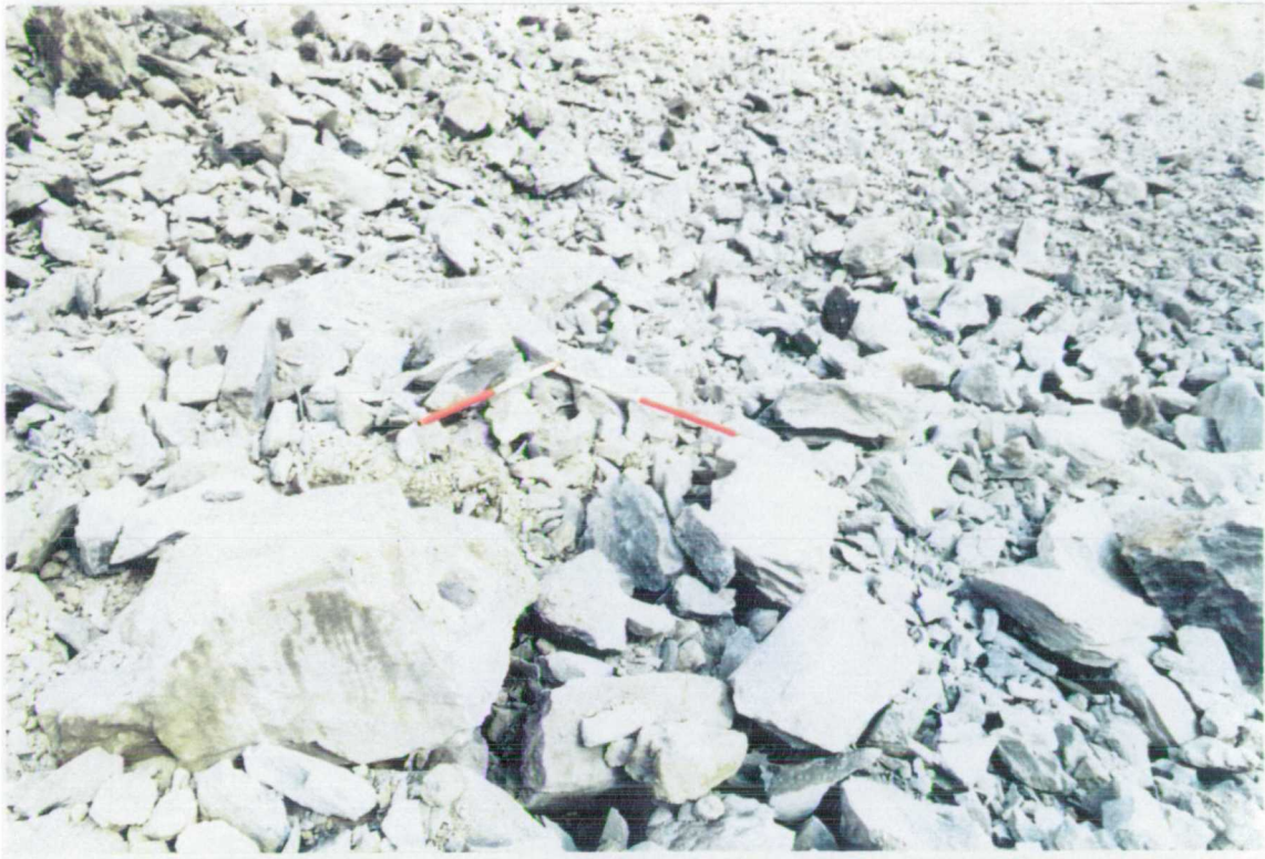
Fig. 7.9 A typical blastpile photograph, B1-1 taken from the A5 site (scale bar: 50 cm division; note, the scale bars form a right angle and this enable a correction to be applied to the photographic data)
