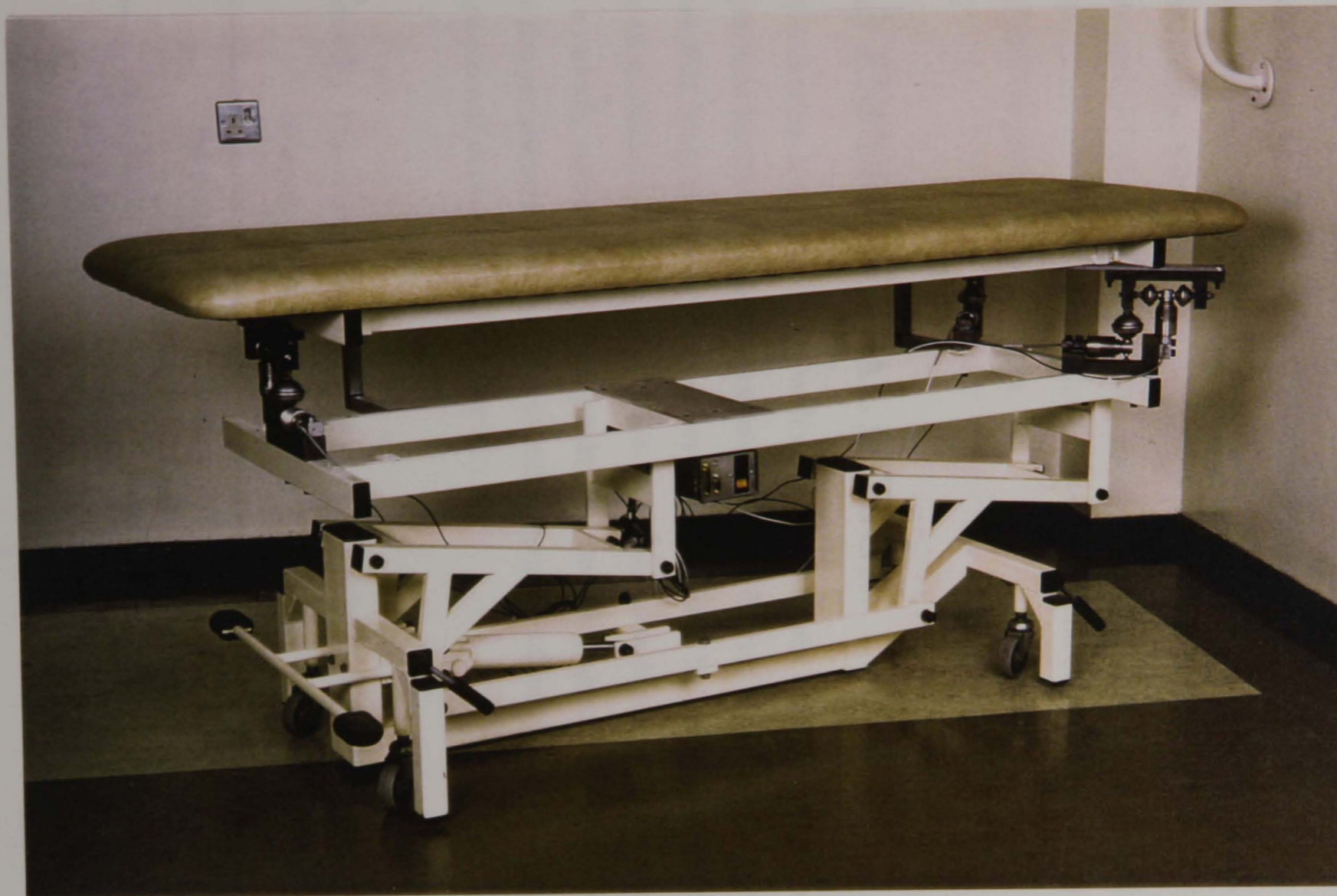
Figure 9-2: The instrumented couch illustrating the increase in height resulting from the inclusion of load cells within the frame
