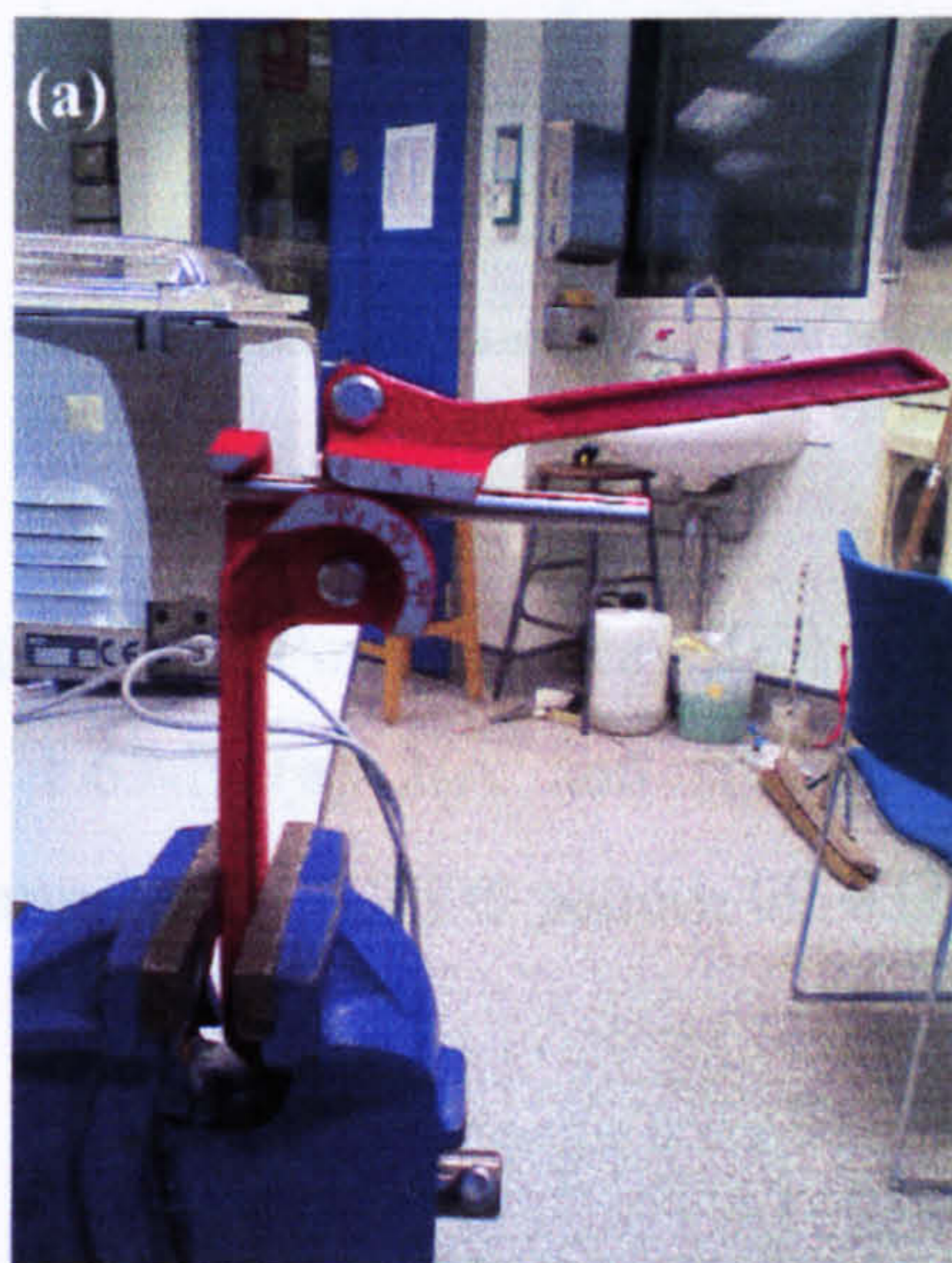
Figure A-4 3/8 th inch 316L Swagelok pipe connecting the 3/8 th cross-piece to cooler (a) when placed in the pipe bender and (b) bent to give a 90-degree angle.
