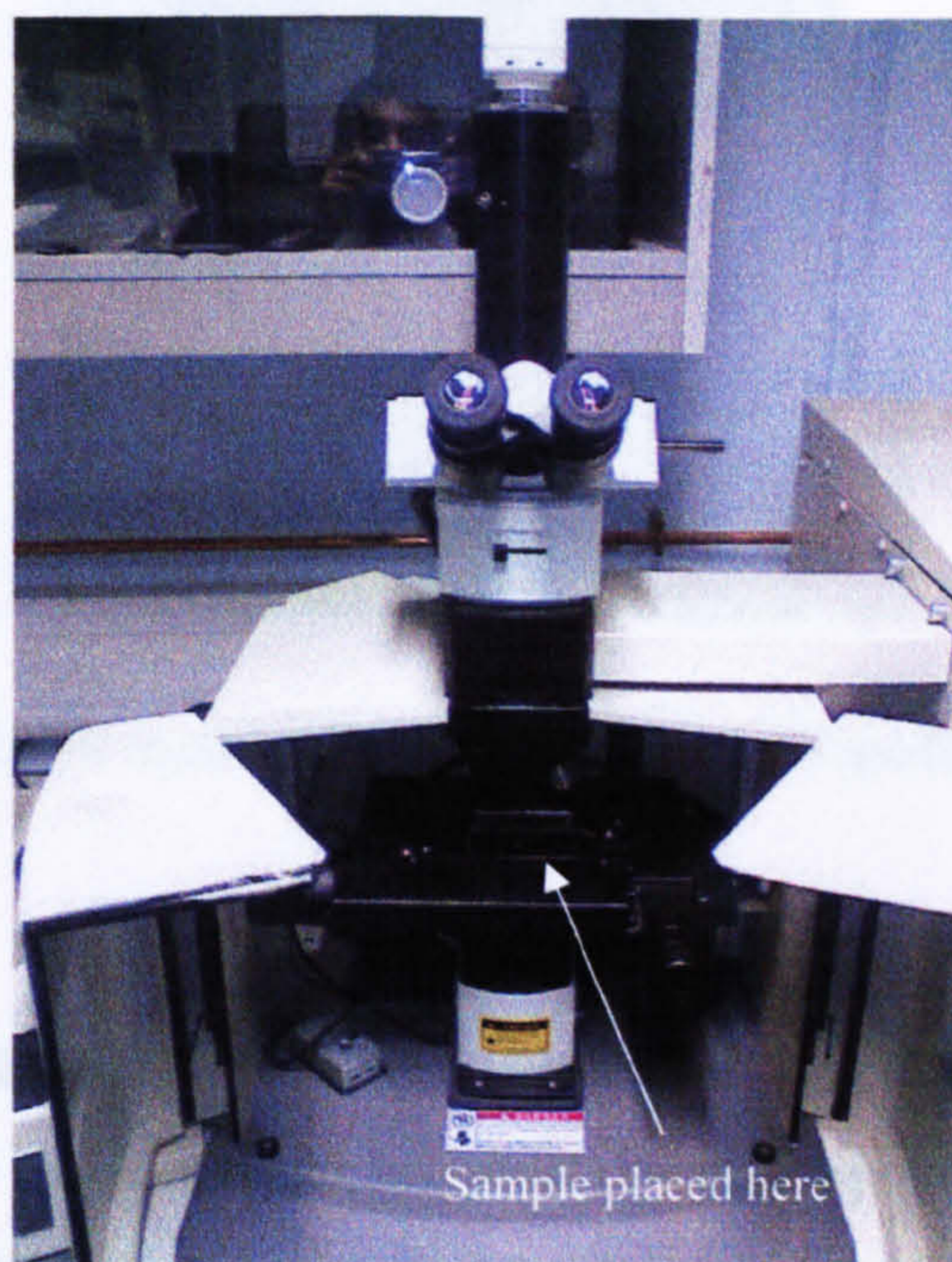
Figure 2-19 The microscope compartment of Nicolet Alpha Dispersive Raman Spectrometer.
