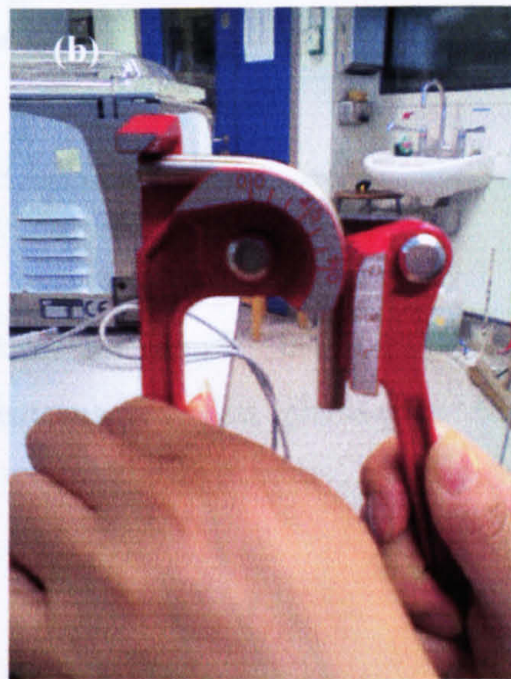
Figure A-4 3/8 th inch 316L Swagelok pipe connecting the 3/8 th cross-piece to cooler (a) when placed in the pipe bender and (b) bent to give a 90-degree angle.
