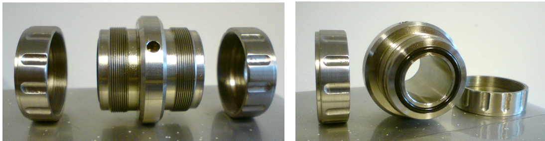
Figure 39 – Final manufactured air-tight sample chamber composed of a stainless steel 316L body and Viton® ‘o’ring seal. Left: exploded side view of chamber, Right: view of o-ring embedded with in stainless steel body.
