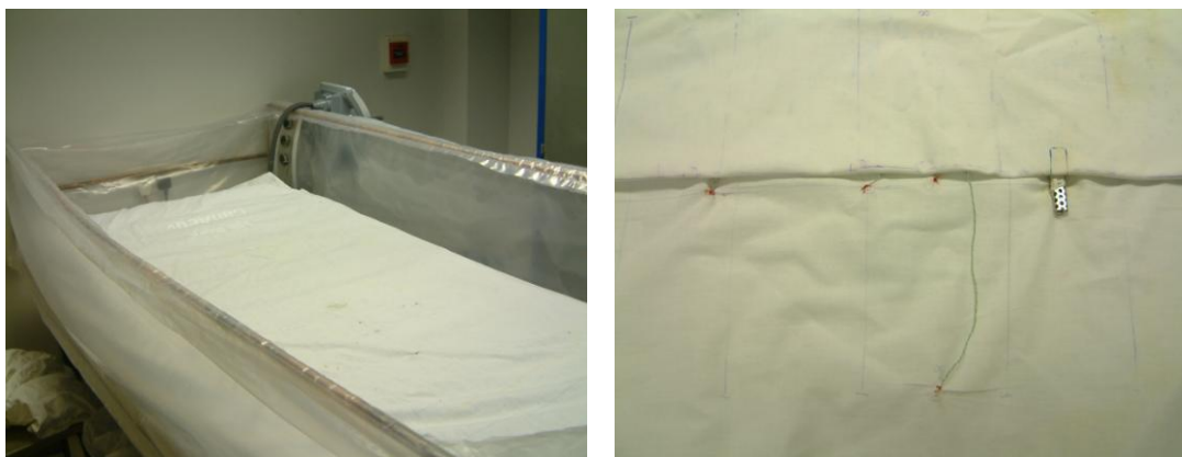
Figure 7 - 9 Left: test arrangement of ClinActiv mattress into the environment chamber. Right: Standard cotton bedding material, doubled to protect the interface sensors.
