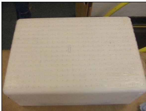
Figure 7 - 6 Human Body analogue with an embedded sweating system made of perforated Tygon® tubing. This surface was touch at the mattress interface in experiment.
