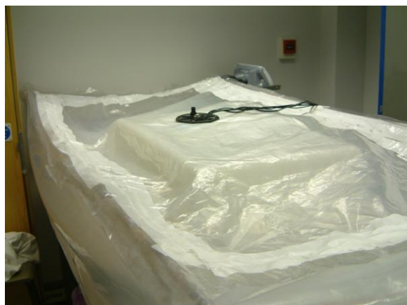
Figure 7 - 10 Enclosed environmental chamber with mattress and human analogue.
