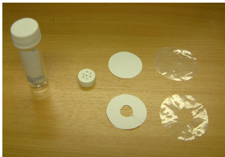
Figure 5 - 1 Image of the materials used to collect and store sweat. From left to right, the screw-capped plastic 30 mL conical bottomed tube, separators with drilled holes, and both circular and annular shapes of sweat collection pad and polypropylene plastic film over the top during the measurement.
