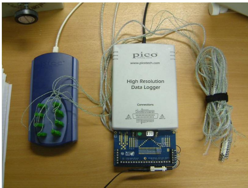
Figure 7 - 4 Photo display all humidity and temperature sensor system.
