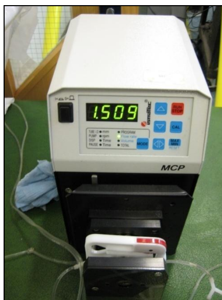
Figure 7 - 7 The peristaltic pump used to simulate sweating by delivering heated water to the body mattress interface.
