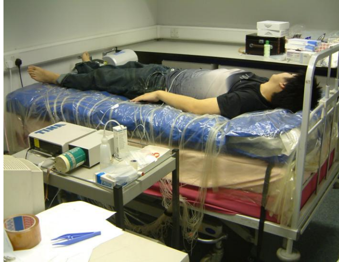
Figure 5 - 4 Images showing a subject lying prone on the APAM support with measurement sensors attached.
