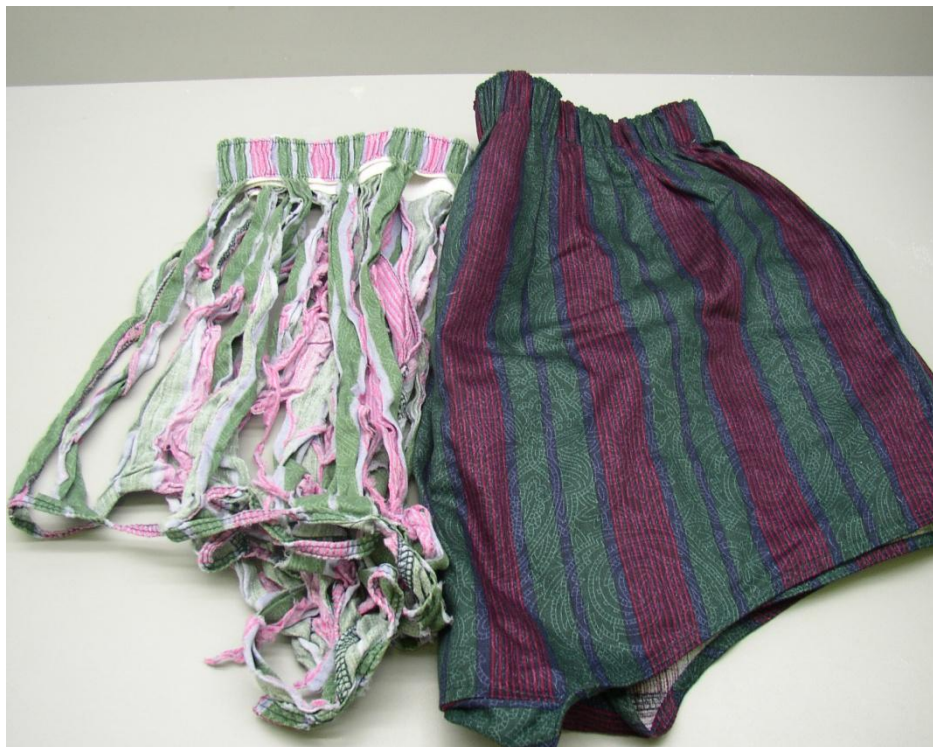
Figure 1. Marks & Spencer's Boxer Shorts (after and before 20 repeat washes at 50 °C)
