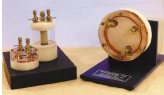
Figure 7: Basic make-up of a rotating-wall vessel reactor taken from (Hammond and Hammond 2001) and originating from the article of (Goodwin et al. 1993a). Basically the bioreactor from the left-hand side is attached horizontally to the end-piece on the right-hand side. Rotation is relative to the horizontal axis; rotation in the spinner flask from the preceding section is along the vertical axis.
