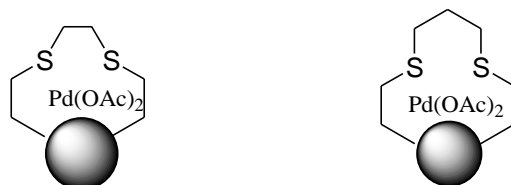
Figure 3.3 Catalysts silica-60-C 2 -Pd(OAc) 2 ( S loading 0.56 mmol/g , Pd loading 0.26 mmol/g) and silica-60-C 3 -Pd(OAc) 2 ( S loading 0.50 mmol/g , Pd loading 0.42 mmol/g).
