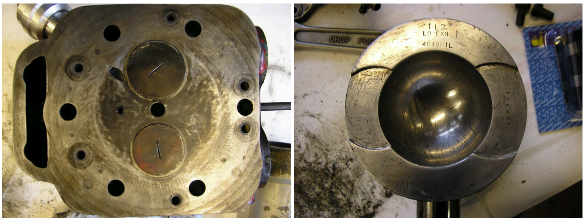
Figure 120: Gardner 1L2 cylinder head (left picture); and piston (removed from engine block) after cleaning (right picture)
