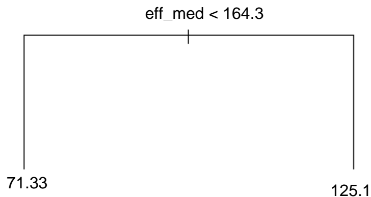
Figure 5.9. The pruned regression tree for CSM-derived erosion thresholds only has one explanatory variable, median effective particle size with a node at 164 \mu\text{m} (RMSE = 62.79)
