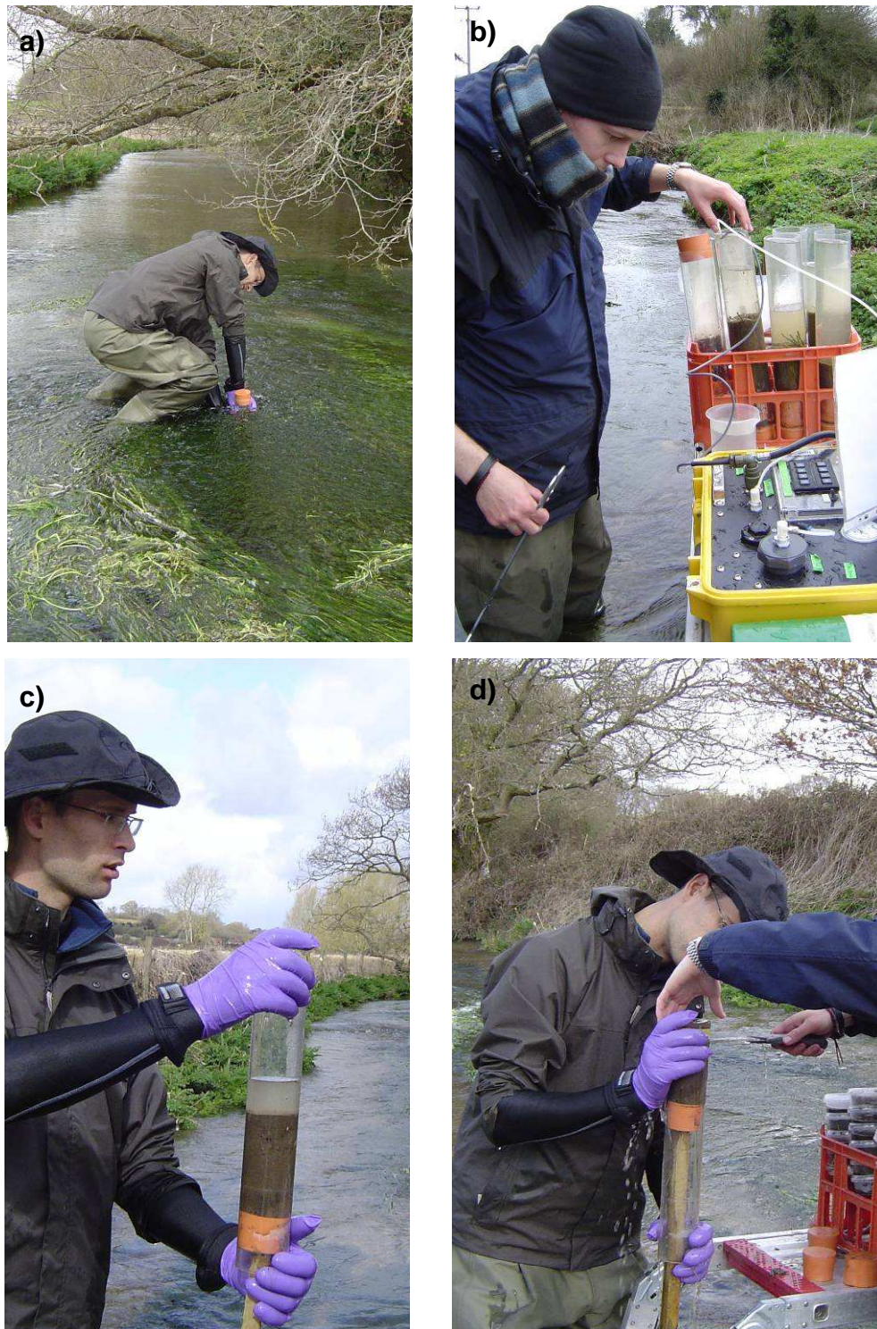
Figure 3.8. Field sampling in the Bere Stream, March 2009, (a) coring, (b) measuring erodibility with the CSM, (c) extruding the core using a plunger, and (d) collecting the top 3cm of sediment.
