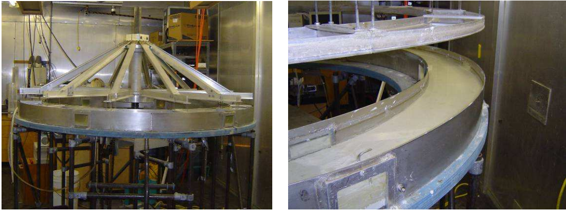
Figure 6.2. The annular flume at the National Water Research Institute, Environment Canada. The flume measures 2 m in external diameter and has a channel width of 20 cm. Water flow is generated by a rotating lid that is lowered onto the sediment surface.
