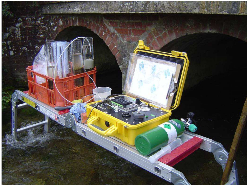
Figure 3.4. The cohesive strength meter (CSM) being used in the Bere Stream. The yellow case is the main unit with computer and a water tank pressurised by the green air cylinder. The pressurised water is transported within the white tubing to the grey test unit within the core tube. A jet of pressurised water is fired downwards within the test unit towards the sediment surface, and resuspension is monitored by a transmissometer.
