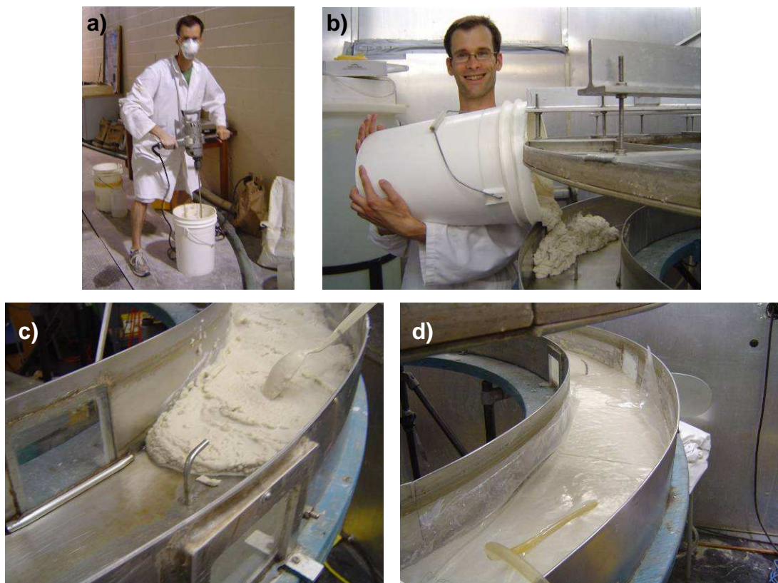
Figure 6.1. Preparation of the sediment mixtures for use in the annular flume calibration experiments. (a) Sediment mixing using a mortar mixing drill, (b) transferring the sediment to the flume, (c) spreading and levelling the sediment in the flume, and (d) filling the flume.
