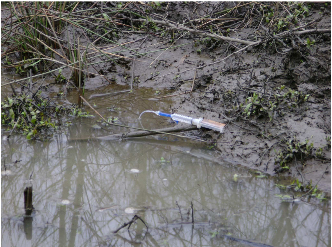
Figure 7.5.4: Rhizon sampler attached to a syringe via a luer-lock adaptor and vacuum application with a wooden spacer in the syringe's plunger. (photo: F. Sgouridis).
