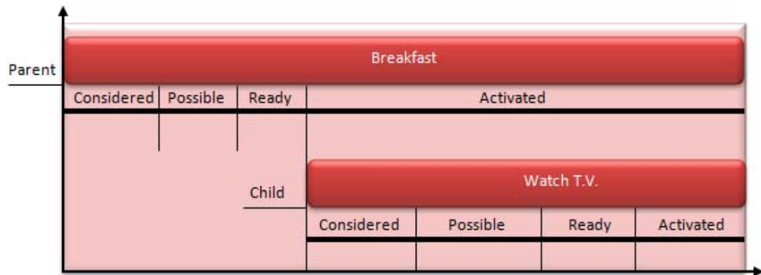
Figure 15 - Parent-Child synchronisation between ADLs in Asbru
