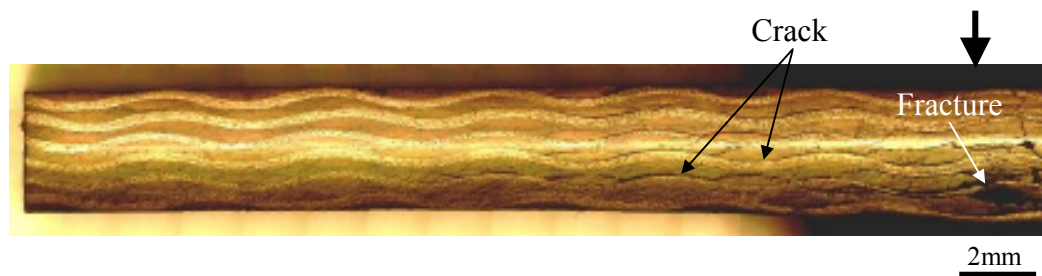
Figure 5.30 Cross-section image of 12J impacted specimen for PE/C (80:20) hybrid veil interleaved epoxy system (Broad arrow indicates impact point)
