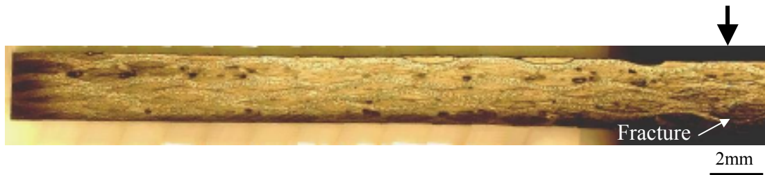
Figure 5.38 Cross-section image of 12J impacted specimen for PA veil interleaved epoxy system (Broad arrow indicates impact point)
