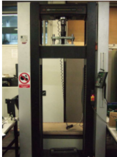
Figure 5.6 Picture of Instron 6025 for compression test
