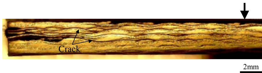
Figure 5.28 Cross-section image of 12J impacted specimen for PE/C (70:30) hybrid veil interleaved vinyl ester system (Broad arrow indicates impact point)
