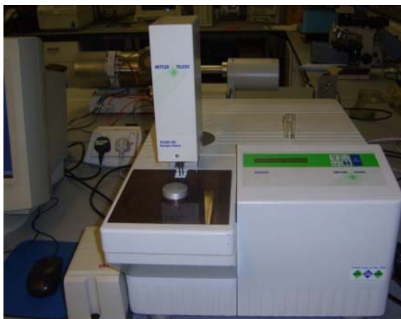
Figure 3.14 Differential Scanning Calorimetry
