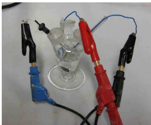
Figure 3. 22 An electrochemical cell with cables connected with the potentiostat: blue connector for RE, red one for WE and black one for CE.
