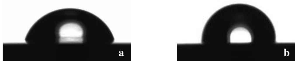
Figure 4. 25 Images of the water contact angles for titanium samples with the APS film prepared with 0.2 v% APTES in: (a) anhydrous toluene and (b) hydrous toluene.
