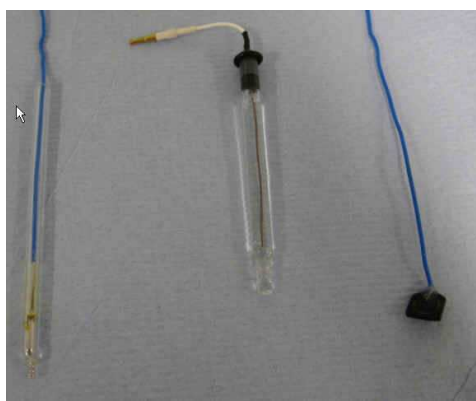
Figure 3. 21 Pt electrode (CE), Ag/AgCl electrode (RE) and graphite electrode (WE), from left to right.
