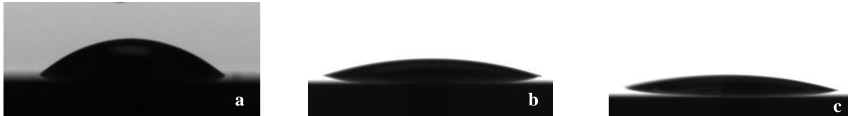
Figure 4. 4 Images for water contact angles of \text{TiO}_x surfaces prepared in Piranha solution (1:1) at room temperature for different immersed time: (a) S_{\text{RT}_5} , (b) S_{\text{RT}_{15}} and (c) S_{\text{RT}_{30}} ( n=6 ).
