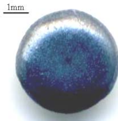
Figure 3.3.19 Optical image of the top surface of the 0.5 mol.% Y-doped BT sample via droplet-doping method sintered at 1380 °C in N 2 flow.
