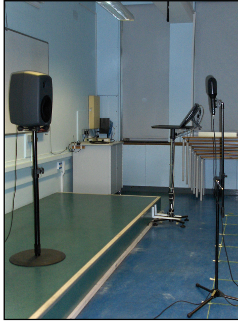
Figure B.1: The Soundfield microphone and Genelec speaker during measurements in the classroom.
