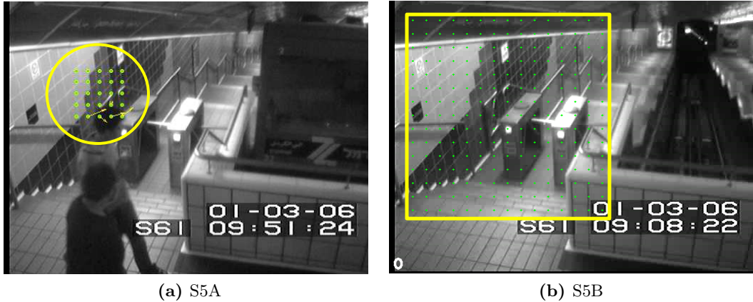
Figure 4.5: Sample frames of sequence S5 depicting a scene from the exit of an underground train station and the selected ROI: (a) S5A for a single detector, (b) S5B for the multi-detector framework.
