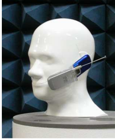
Figure 2.1: Realistic human body phantom for on-body measurements [27]
