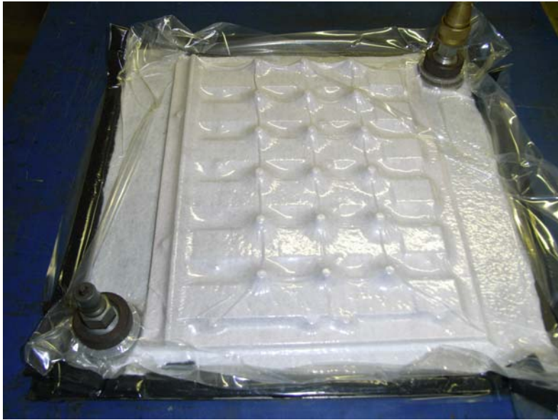
Figure 4. 4 DLJ bonding manufacture using jig and vacuum bag
