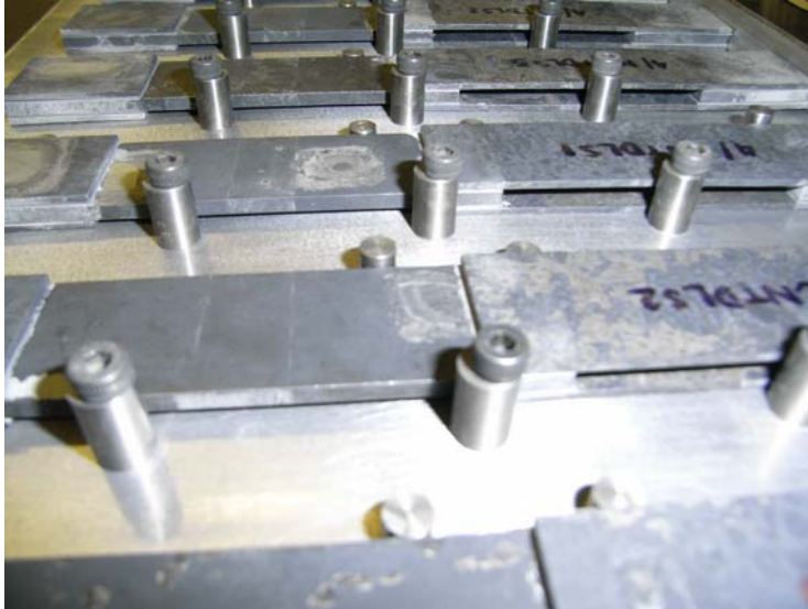
Figure 4. 3 A jig used for DLJ's manufacture
