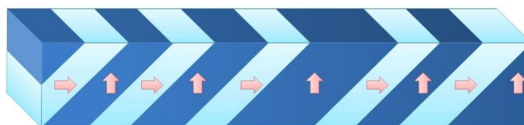
Figure 2.9: Illustration of MSM Sick with martensitic variants and easy axis (red arrows)
