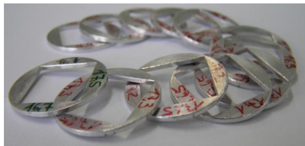
Figure 5.3: Bloc-discs to measure magnetisation at several strain stages
