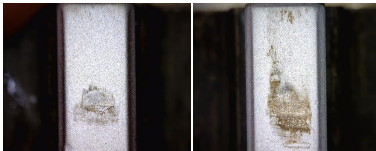
Figure 8.15: Abrasive wear on the core pieces
