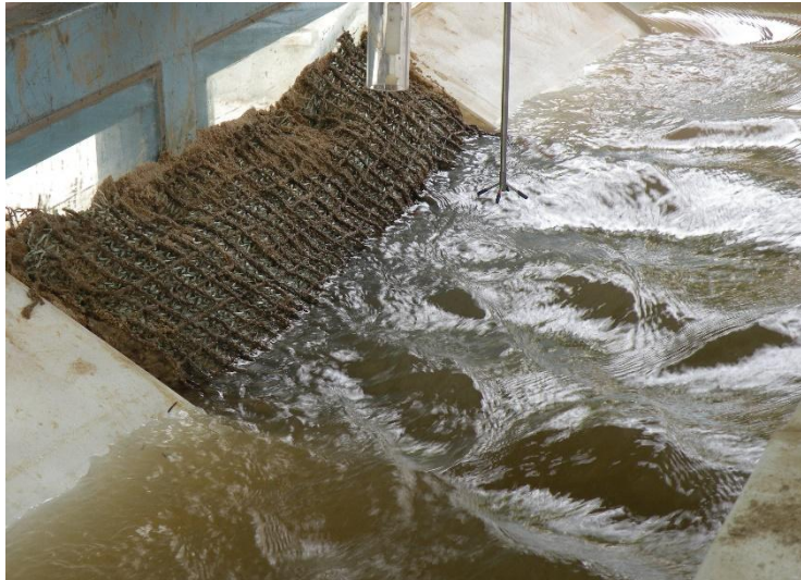
Fig. 2. Acrylic embankment and vegetation mat installed in the channel
