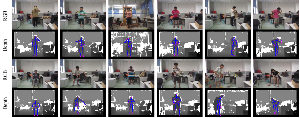
Fig. 8. Snapshots of activities in SYSU 3D HOI set, one sample per class. The rows headed with RGB show the samples in RGB channel and the rows underneath headed with Depth show the corresponding depth channel superimposed with skeleton data. Best viewed in color.
