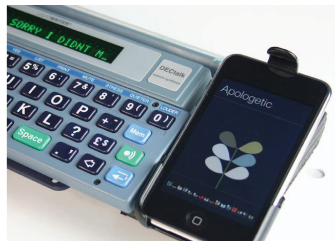
Figure 5. Speech Hedge interface for tone of voice, showing leaves, plants, and a hedge.
