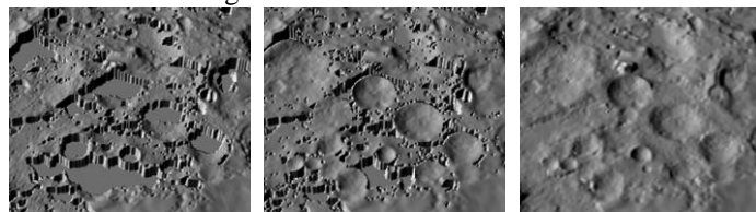
Figure 7: DEM Processing; the original DEM (left), crater filled (center) and fractal hole filled (right)
