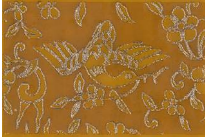
Fig. 5. A 12 mm × 20 mm sample produced for aesthetic purposes. The image demonstrates the visual effects of the nanosecond pulsed laser processing of the nanocomposite. The background and silver outline are processed at the laser energy fluence of 0.3 and 1.1 J/cm 2 , and the number of pulses per spot of 150 and 750, respectively.
